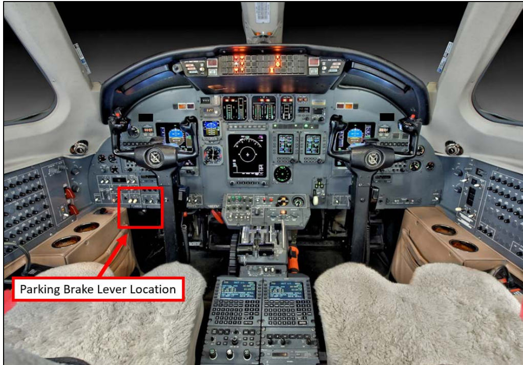
Figure 8: Overview of exemplar cockpit and location of parking brake lever
