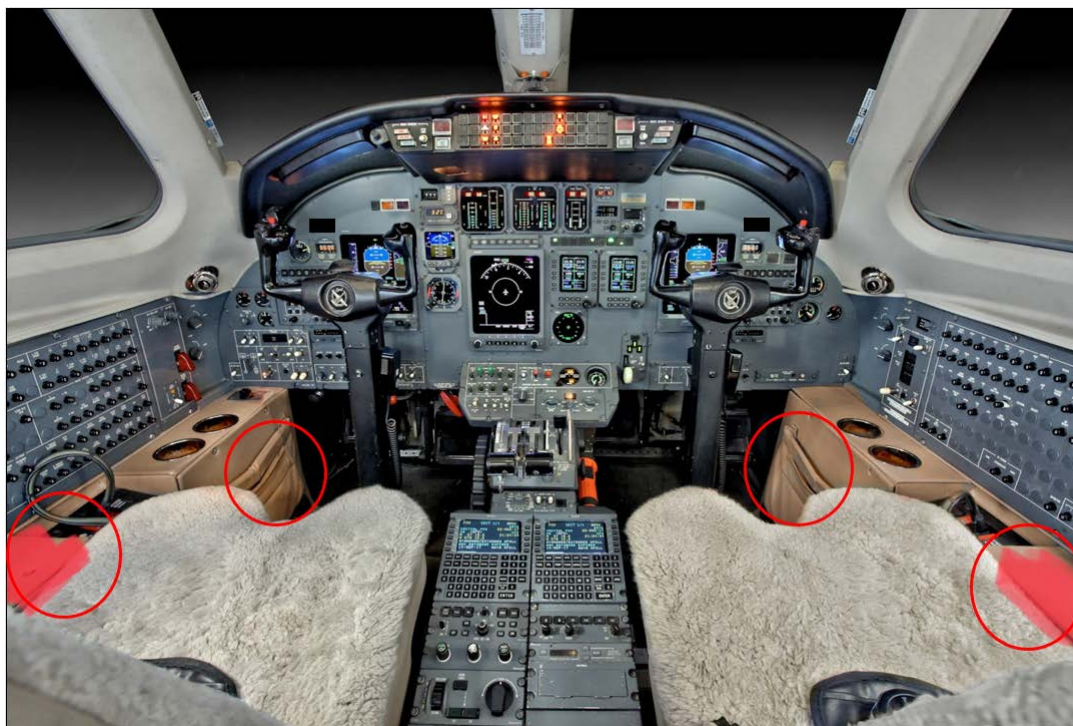
Figure 5: Red circles denoting the common placement of EFB's in the CE560XL cockpit.
