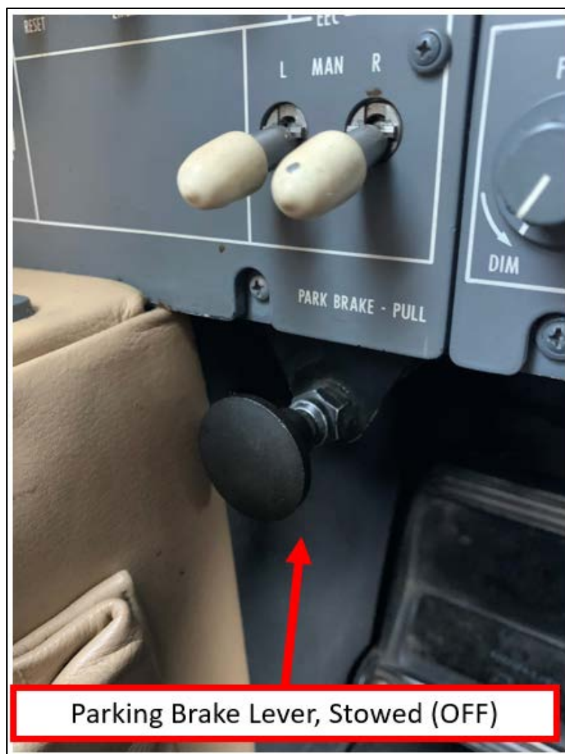
Figure 10: Exemplar parking brake lever, stowed (Off)
