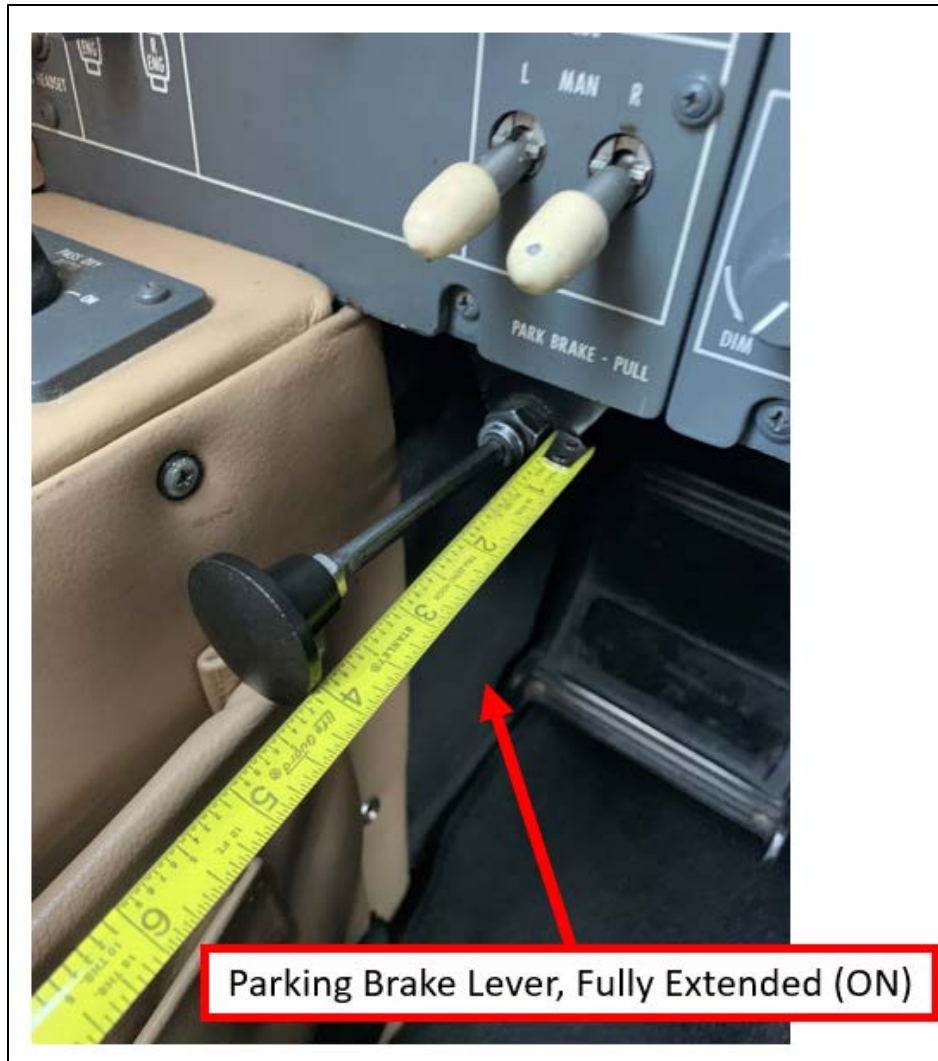
Figure 9: Exemplar parking brake lever, extended (On)
