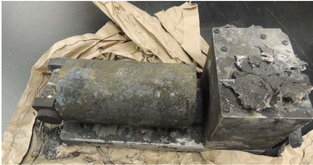
Figure 1. Damaged exterior of flight data recorder
