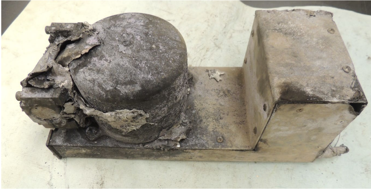
Figure 1. Exterior damage to CVR crash case and chassis
