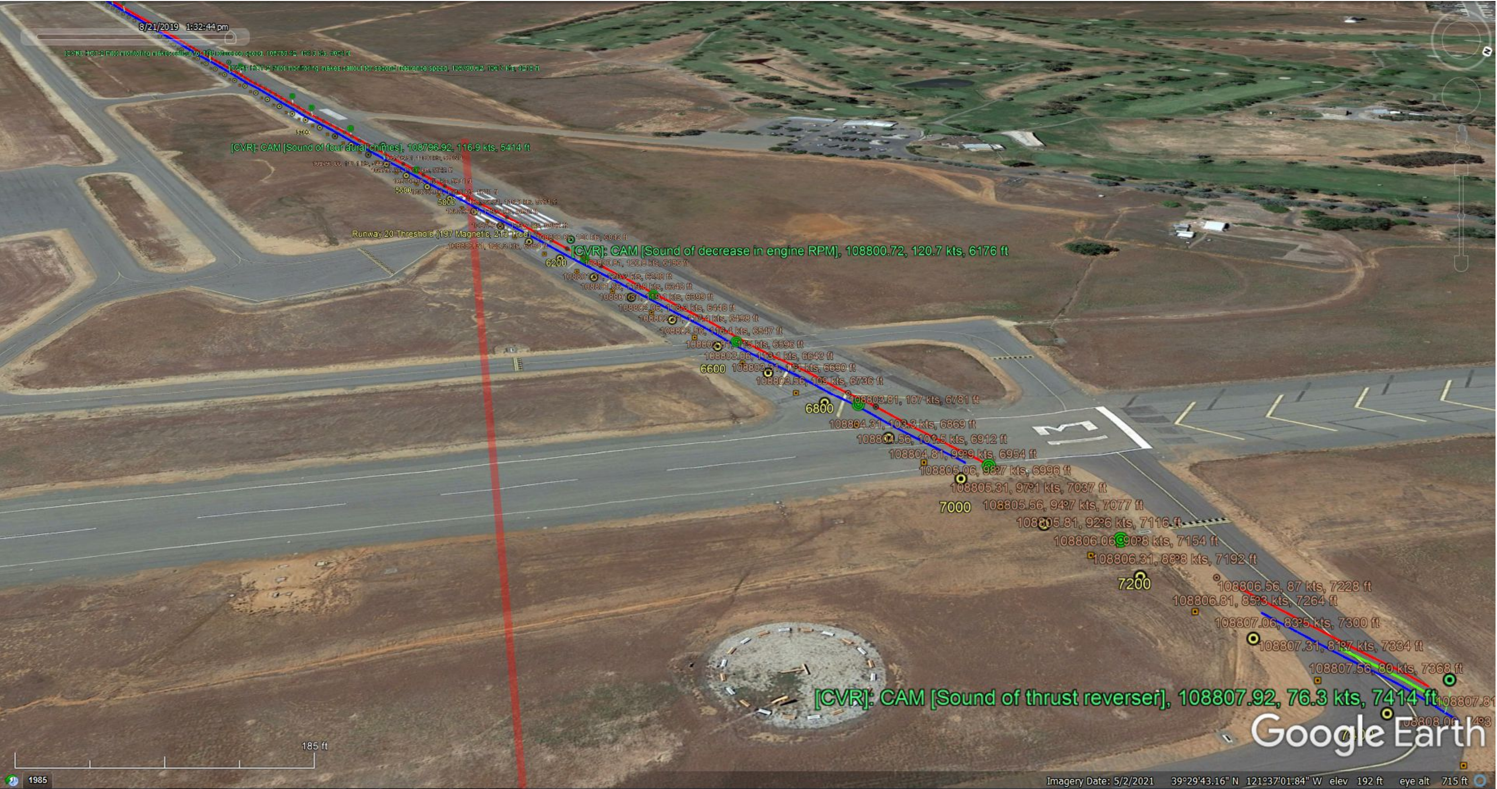
Figure A8.4: N91GY ground track reconstruction, based on FDR, paraphrased CVR, and ADS-B data; tire witness marks; and surveillance camera video evidence. Takeoff rejected.
