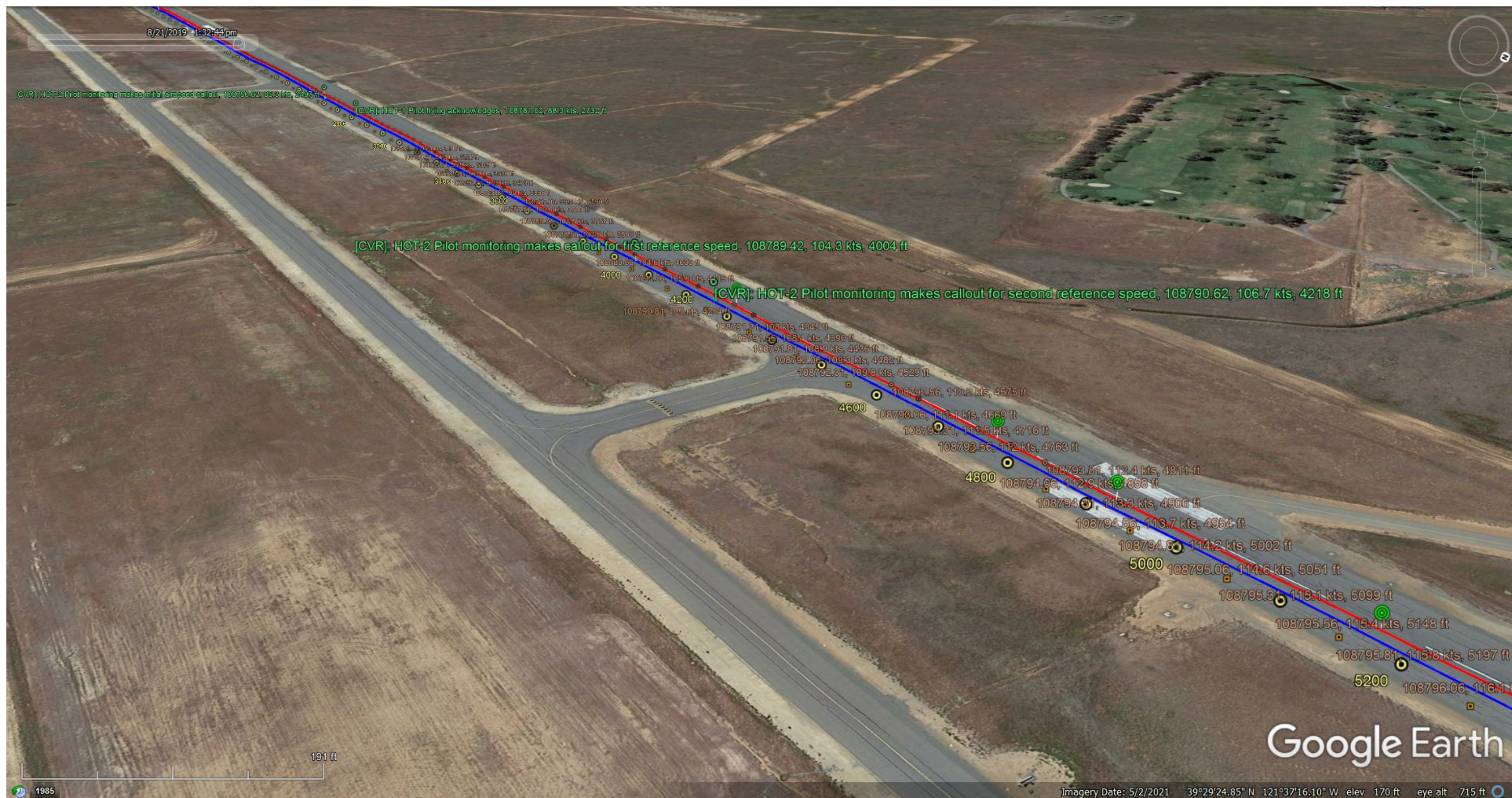
Figure A8.3: N91GY ground track reconstruction, based on FDR, paraphrased CVR, and ADS-B data; tire witness marks; and surveillance camera video evidence. Takeoff acceleration reaches V1 and VR.
