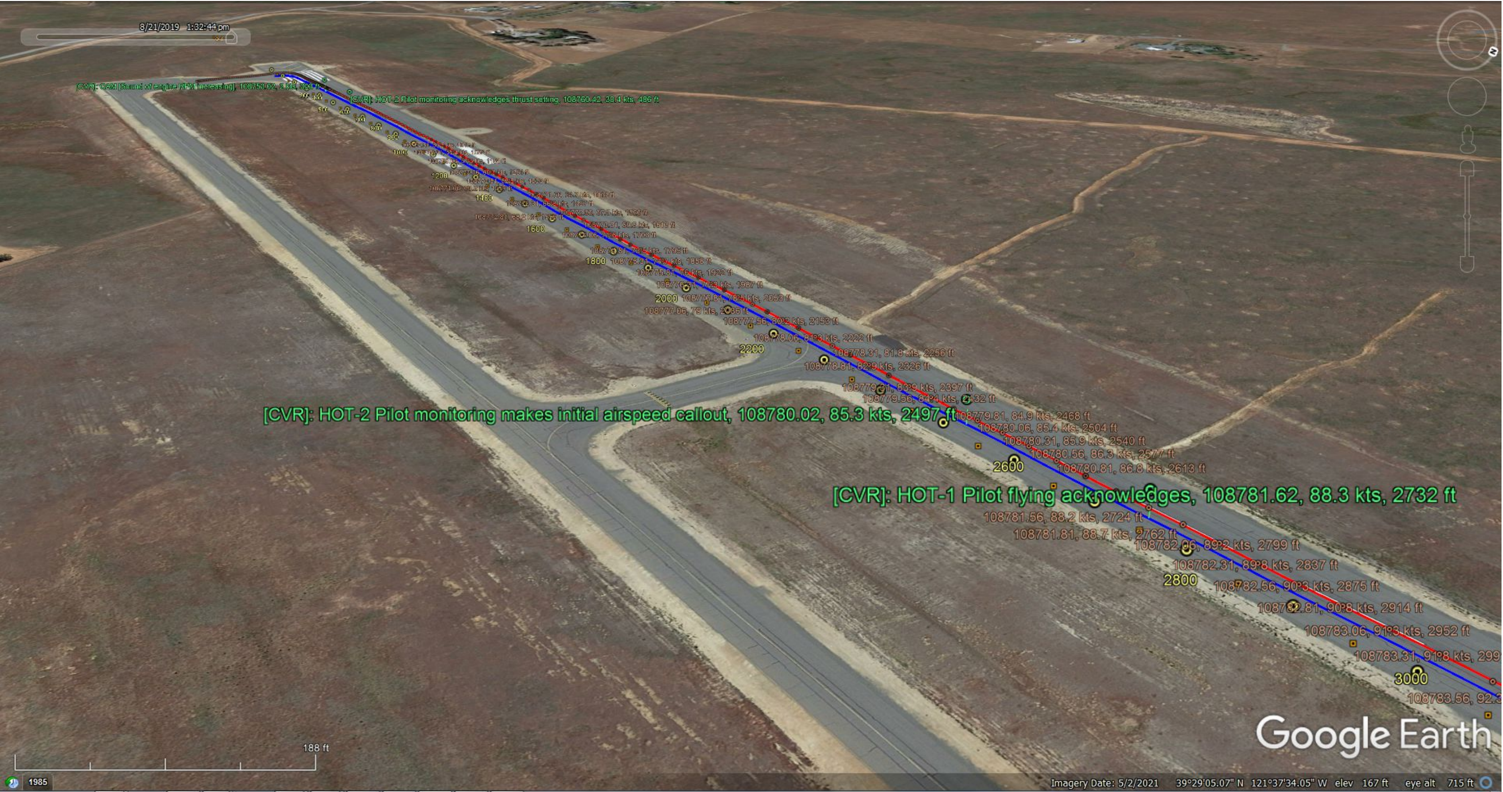
Figure A8.2: N91GY ground track reconstruction, based on FDR, paraphrased CVR, and ADS-B data; tire witness marks; and surveillance camera video evidence. Initial takeoff acceleration period.
