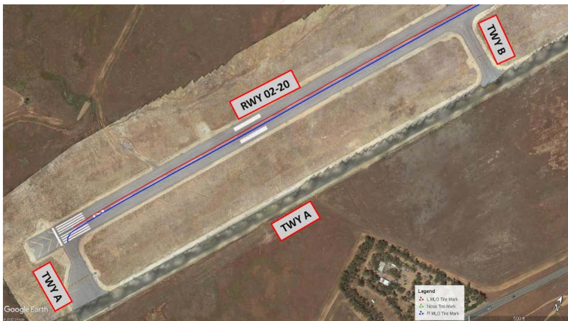
Figure 10 - Tire mark trails from accident site GPS trail at beginning of runway.
