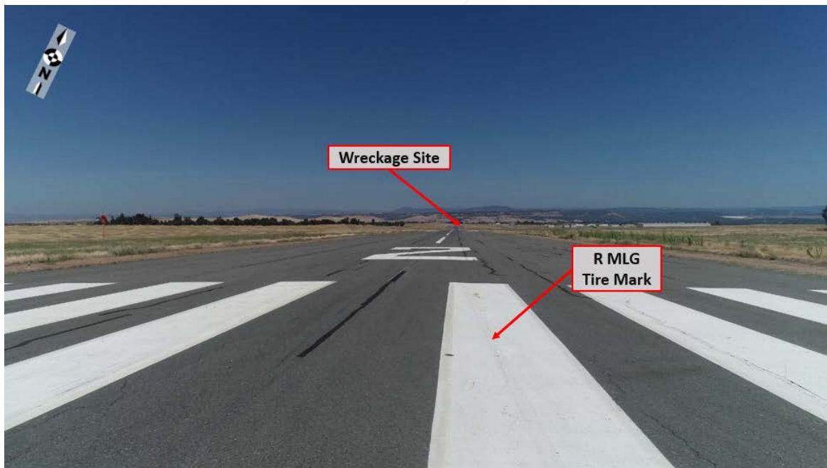
Figure 3 – Runway 02 at start of take-off point with R MLG tire mark
