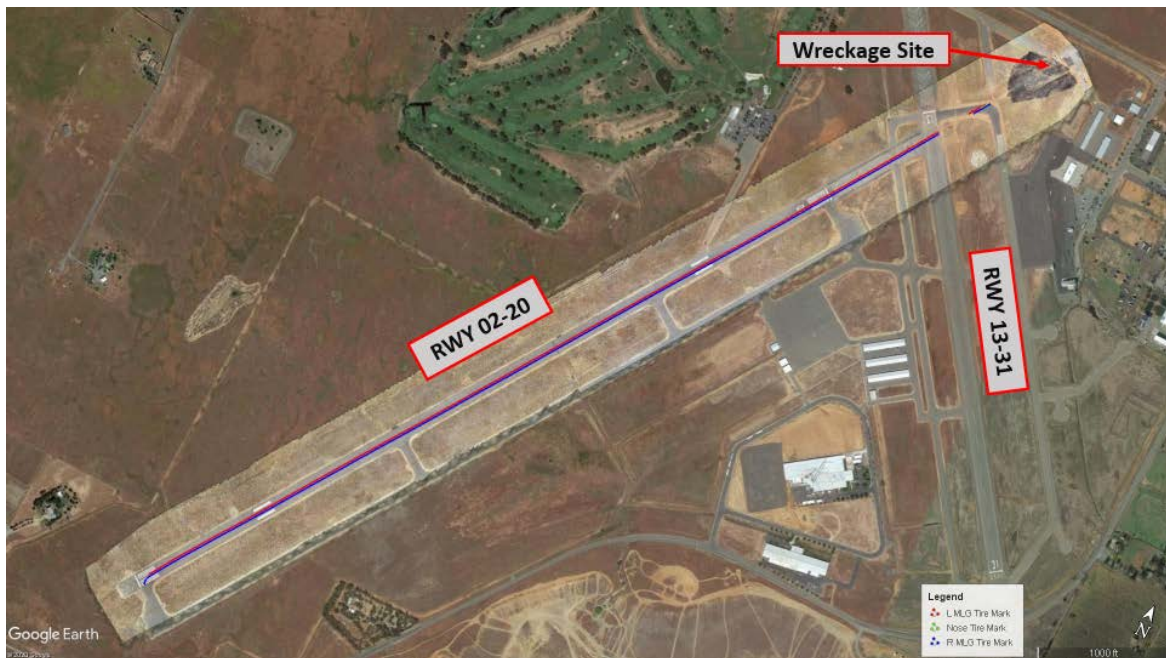
Figure 9 - Tire mark trails from accident site GPS trail.
