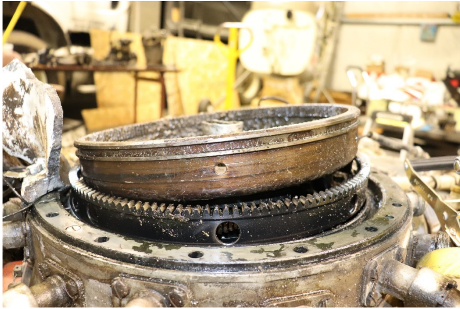
Figure 3. View of nose case gear assumably damage.
