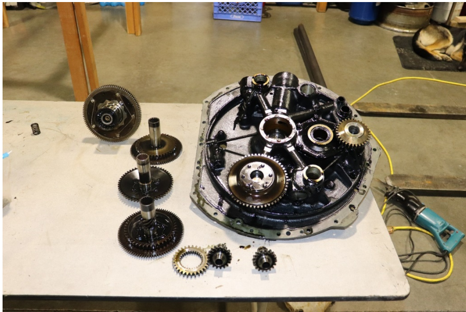
Figure 4. View of accessories case internal components.
