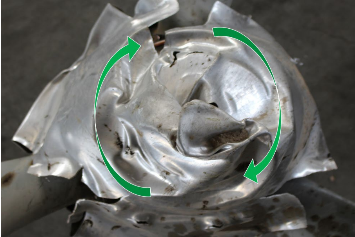
Figure 4: View of rotational forces on propeller spinner.
