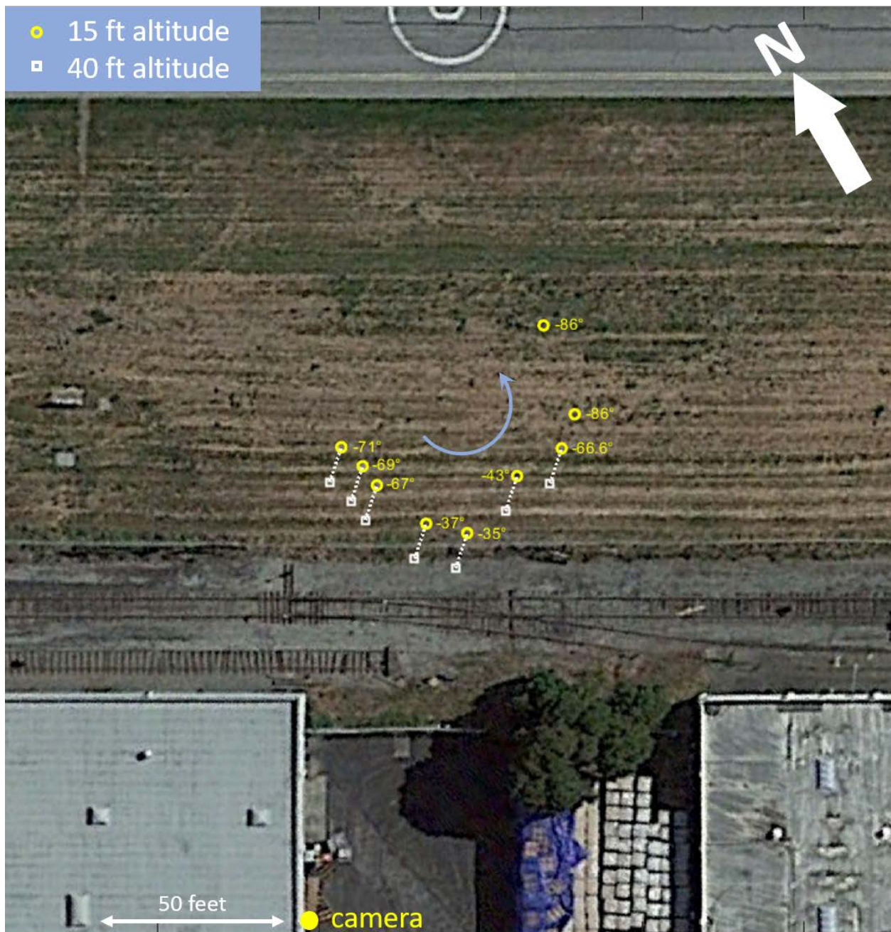
Figure 4. Estimated Helicopter Locations (altitude: 15 feet and 40 feet)
