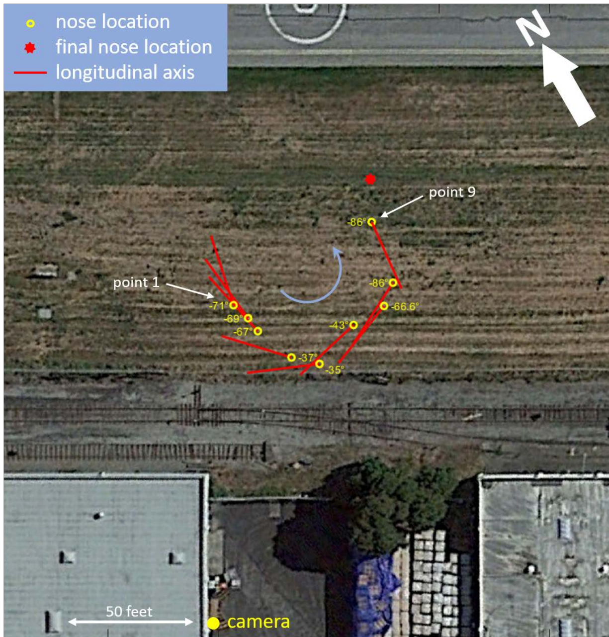
Figure 3. Estimated Helicopter Locations and Headings (altitude: 15 feet)
