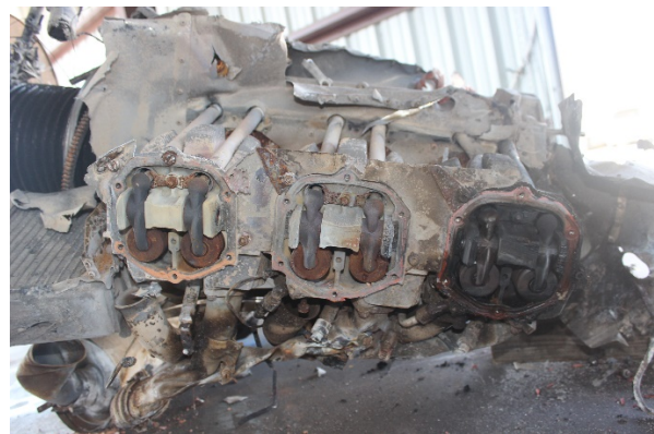
Figure 4. #2, #4 and #6 intake and exhaust valve
