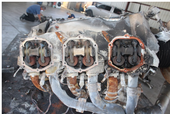
Figure 3. #1,#3 and #5 intake and exhaust valve
