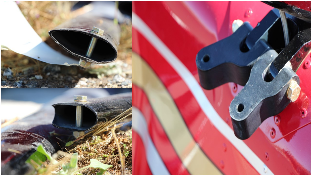
Photograph 2: Left Wing Strut Attachment Fittings
