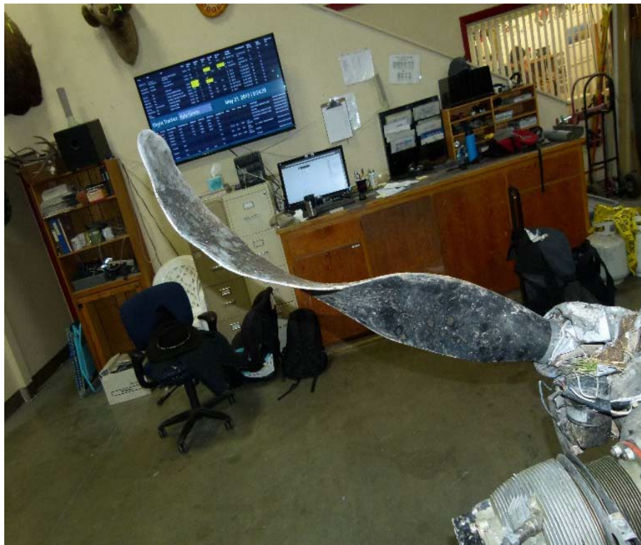
Figure 8 - photo of damaged attached propeller blade
