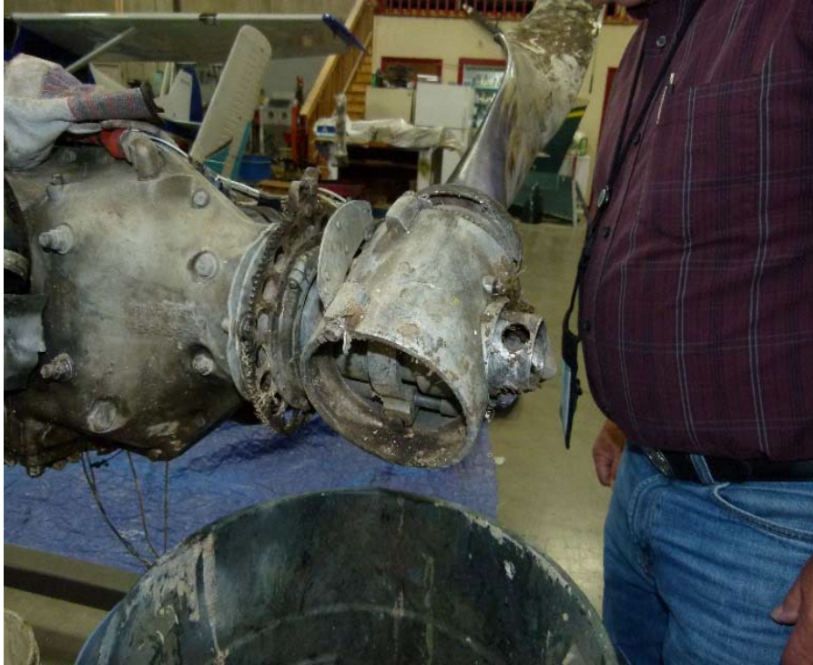
Figure 9 - photo of damaged propeller hub and attached blade
