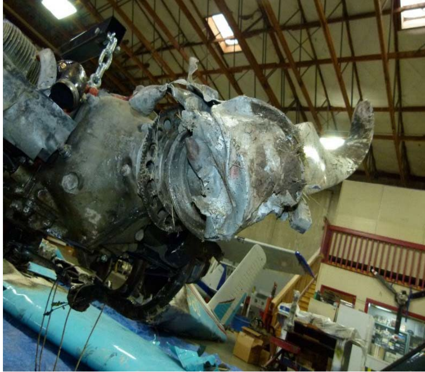
Figure 7 - photo of damaged propeller hub and attached propeller blade
