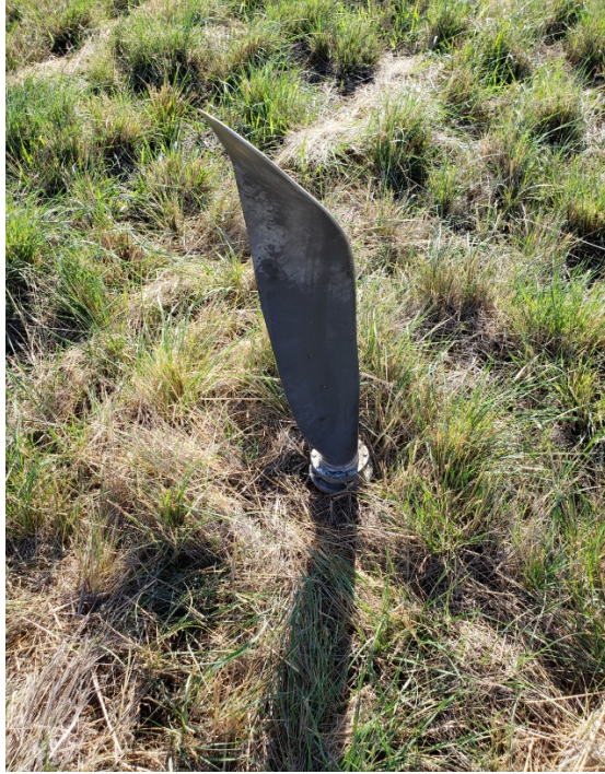
Figure 11 - photo of separated propeller blade
