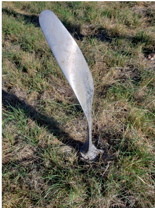
Figure 10 - photo of separated propeller blade
