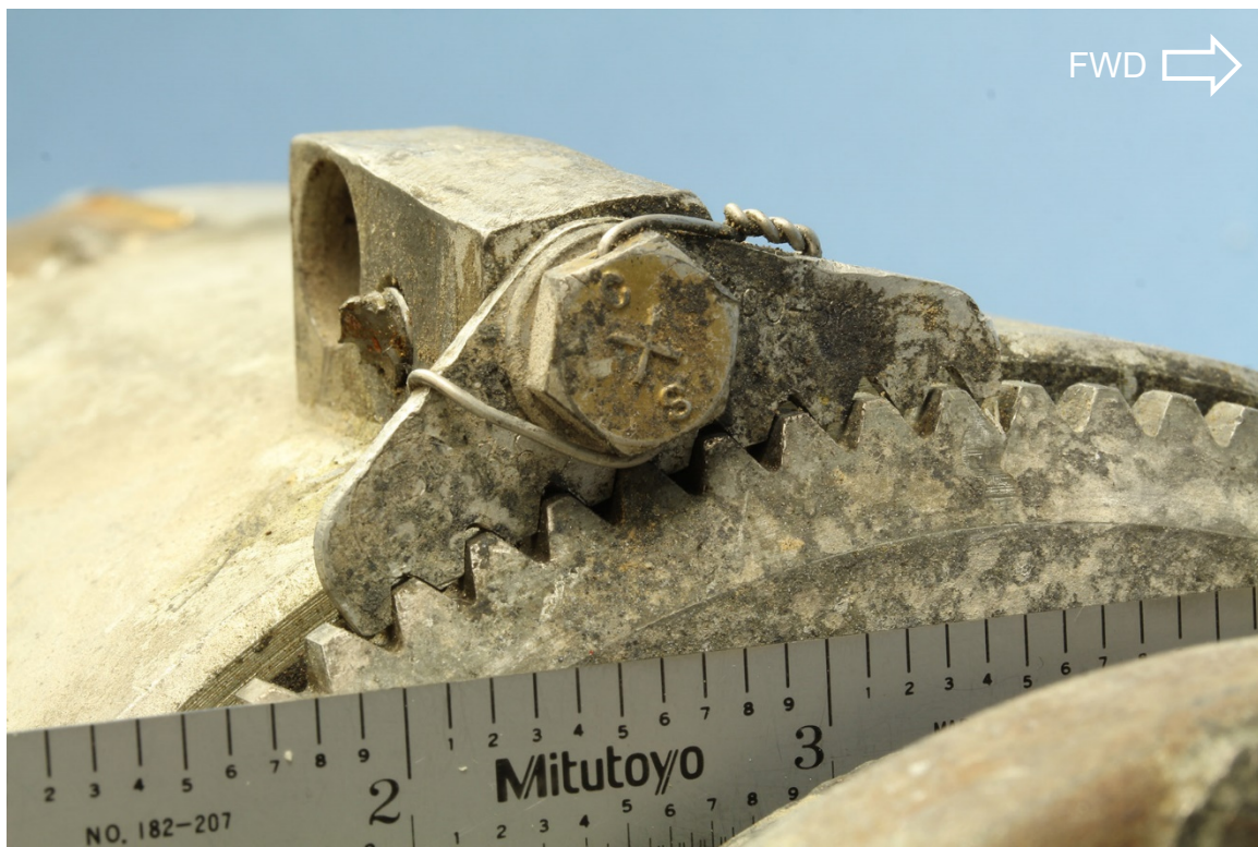
Figure 3 (cont.): c) and d) Images of the two lugs and blade retention nut clips on the intact side of the hub.
