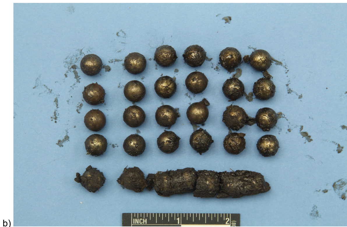
Figure 8: a) Image of one of the thrust bearing upper race fracture surfaces and b) image of the thrust bearings (31 total) in their as-received condition.
