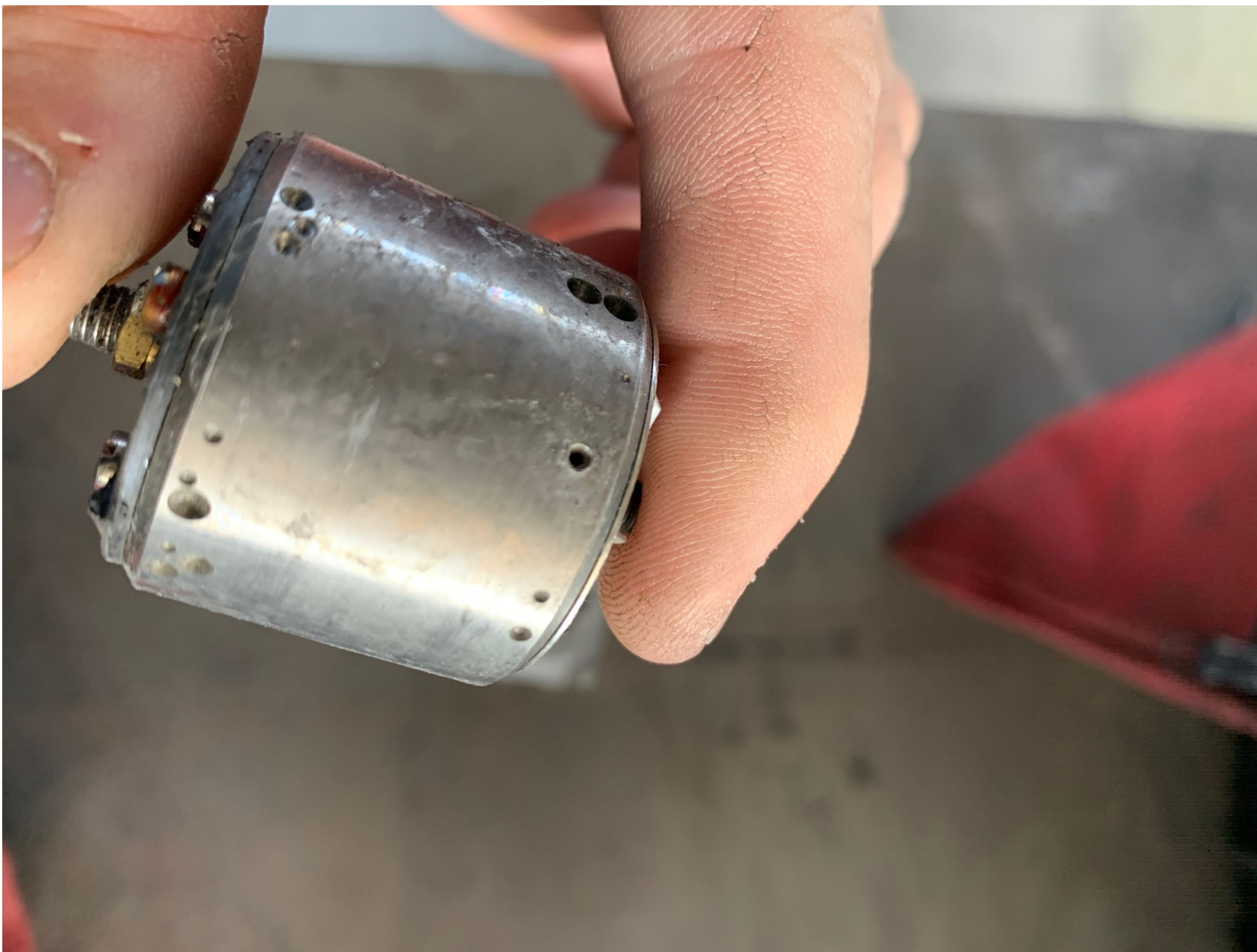
Photo 6 - View of the recovered gyro gimble.
