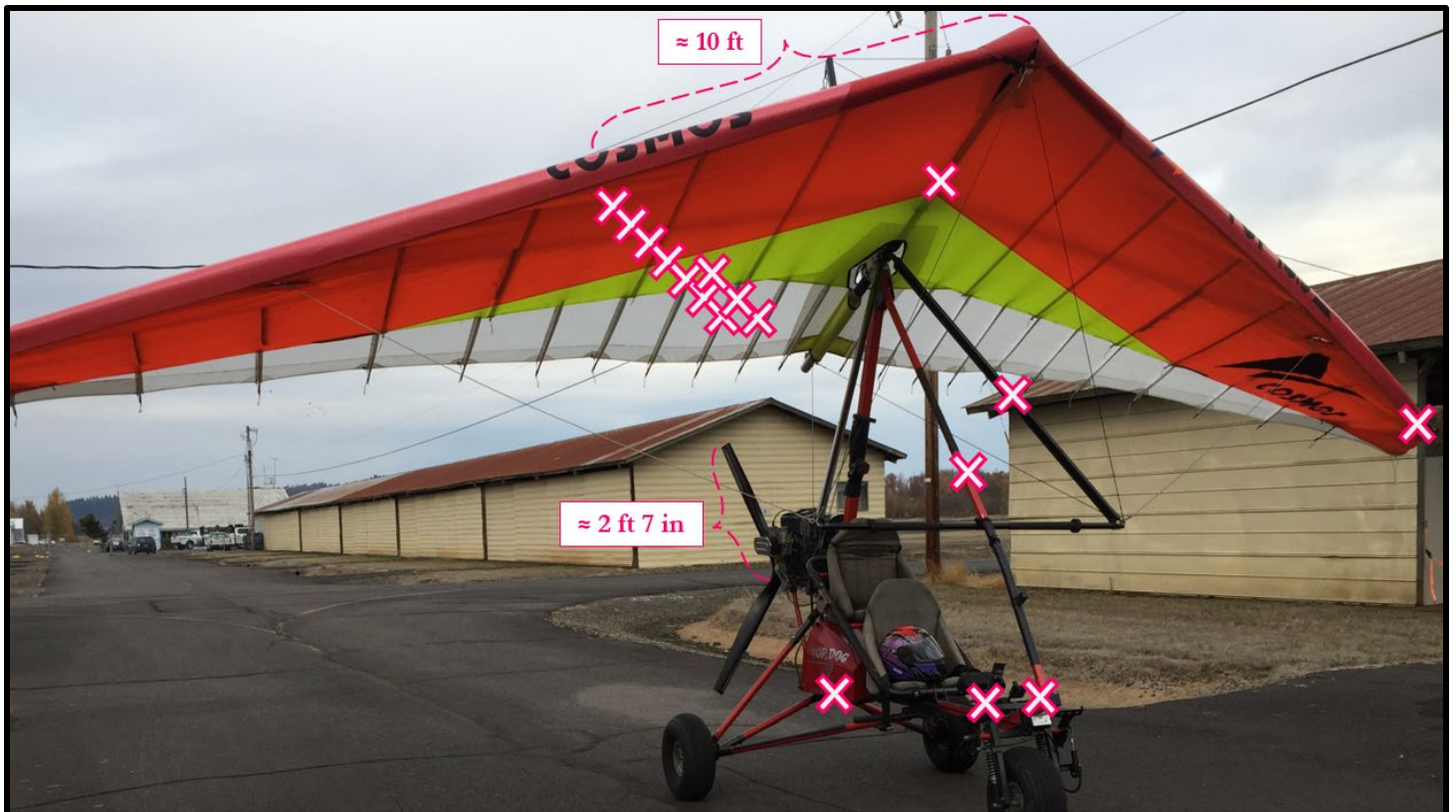
Figure 09: Impact and Damage to Trike Represented by "X" Marks
