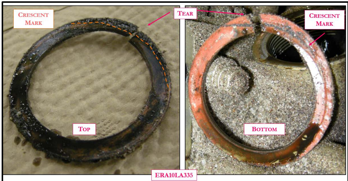
Picture 24: Prior Accident Gasket Showing Impressions/Marks
