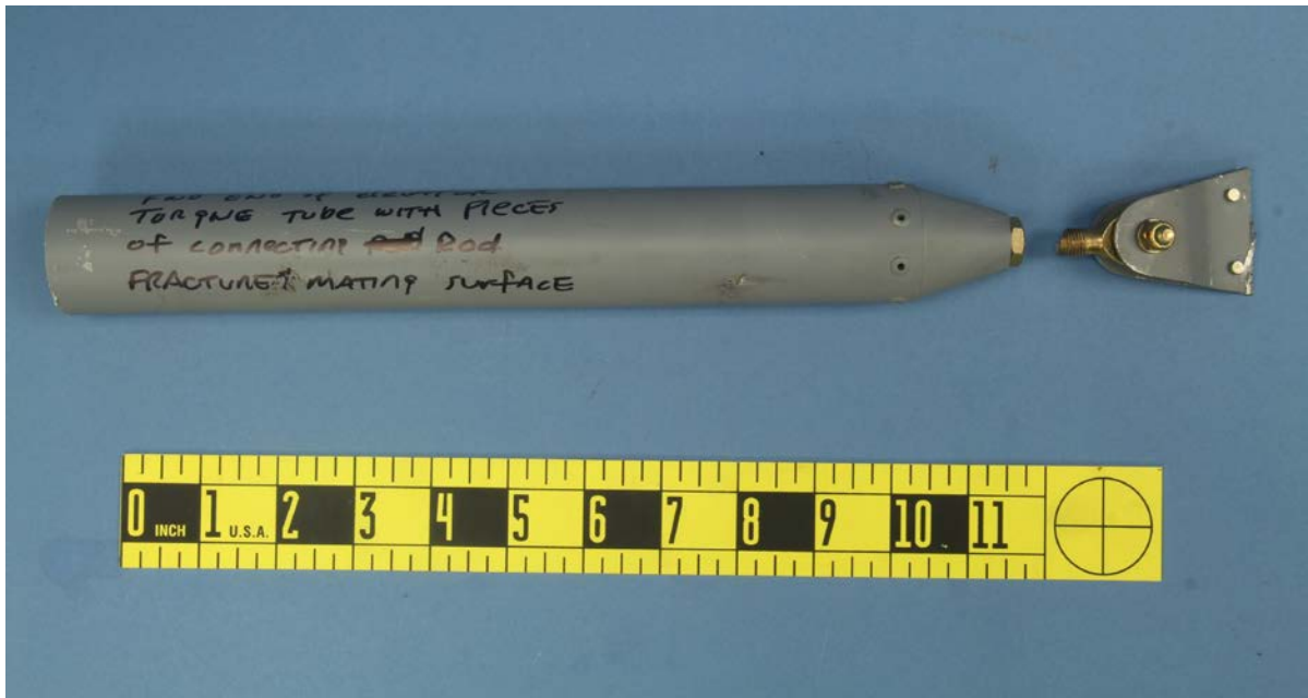
Figure 1: Forward section of elevator torque tube and fractured connecting rod as received.
