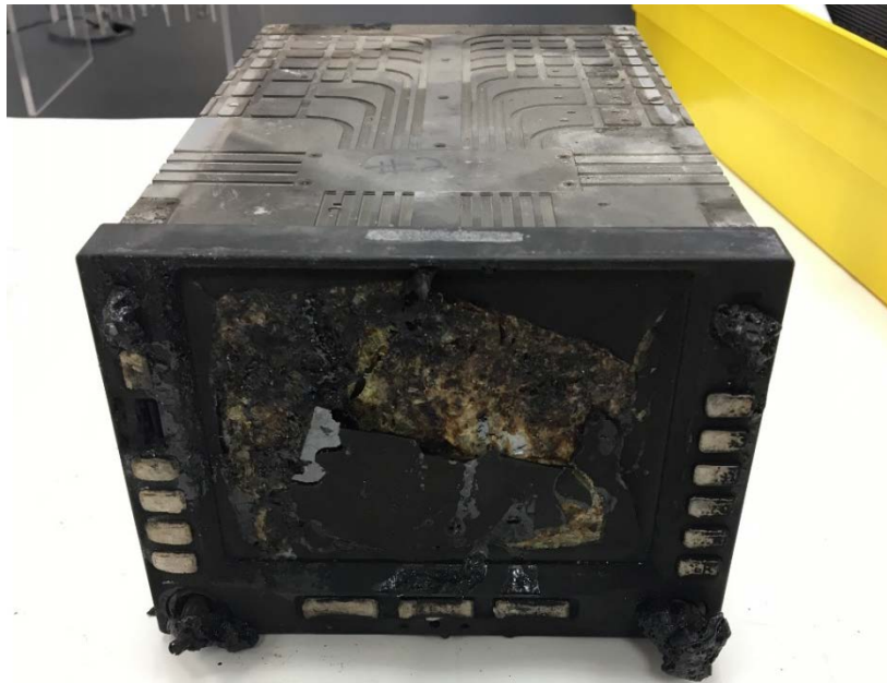
Figure 7. Exterior damage to IFD550.
