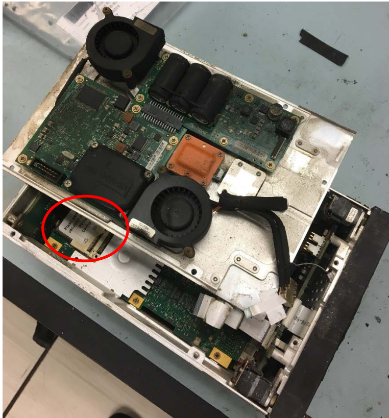
Figure 6. Interior damage and location of CF card.
