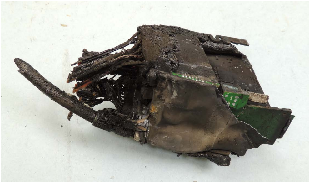
Figure 1. Exterior Damage to Insight G4.
