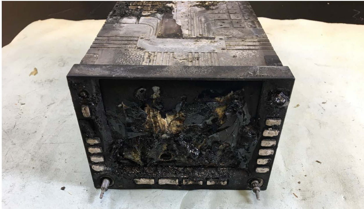
Figure 5. Exterior damage to IFD 540.
