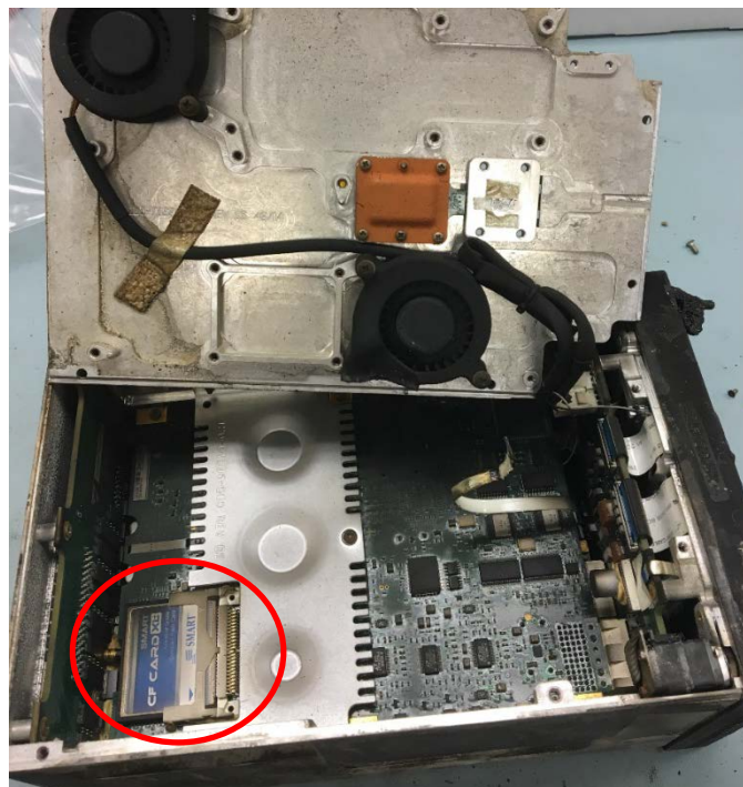
Figure 8. Interior damage to IFD550 and location of CF Card.
