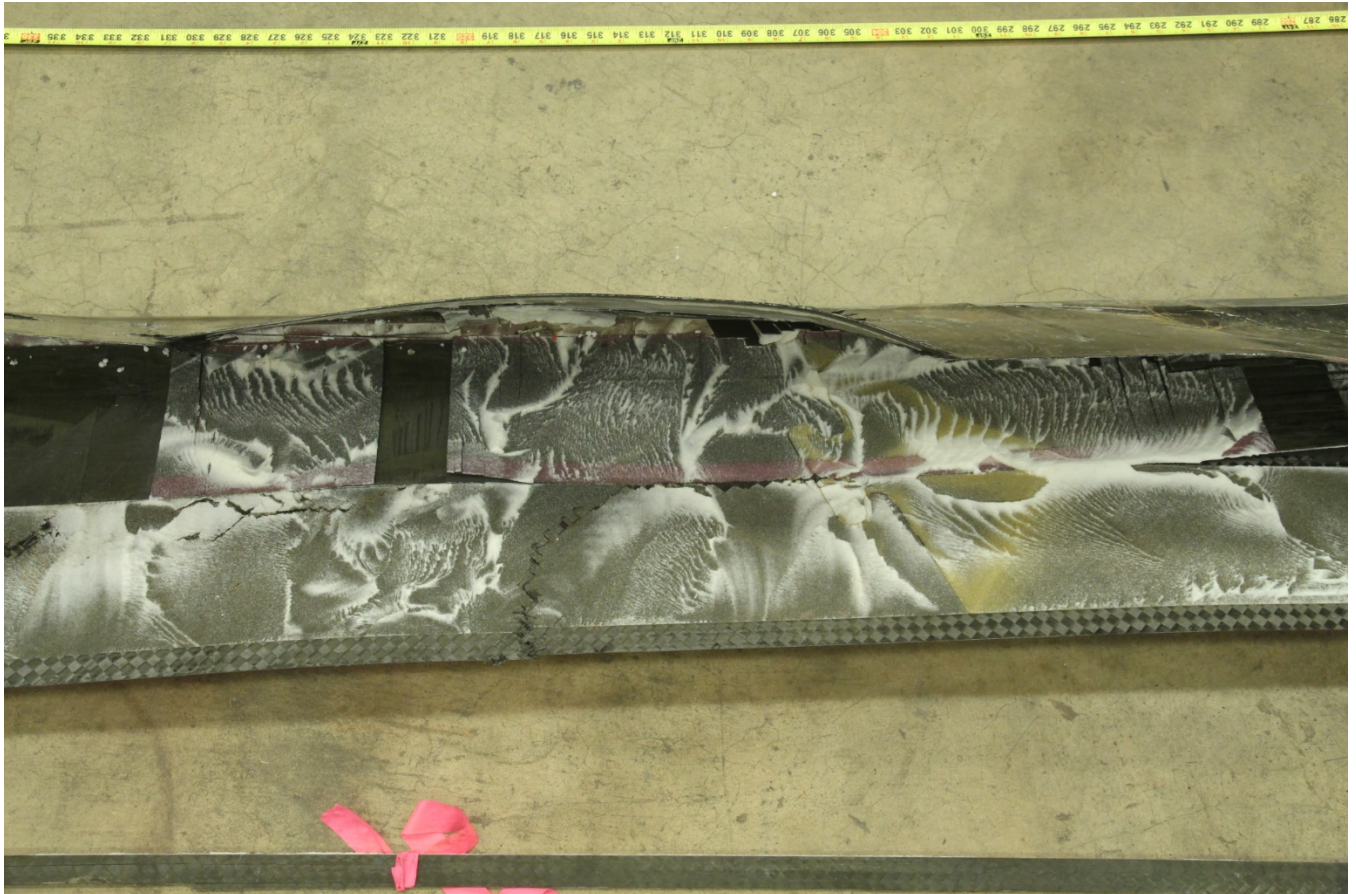
Figure 7 – View of the interior of Blade A by from the trailing edge, showing foam remnants on the interior surfaces.
