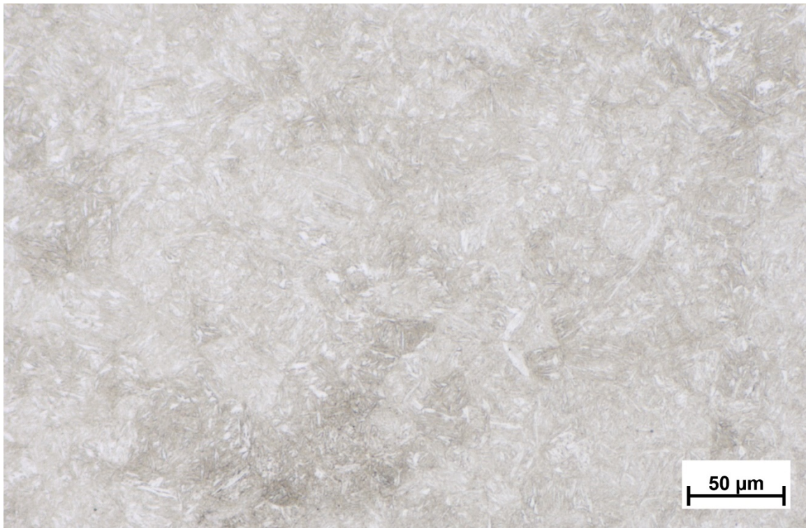
Figure 30 – Bright-field (BF) optical micrograph of the mast microstructure (~500X, etched 2% Nital).
