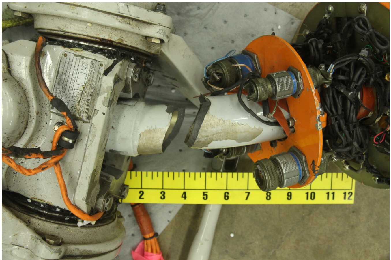
Figure 21 – View of the mating sides of the fractured main rotor mast.
