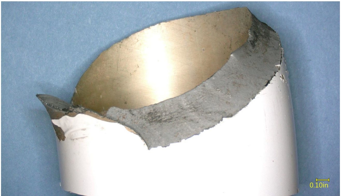
Figure 27 – View of the mast fracture surface, after sectioning.
