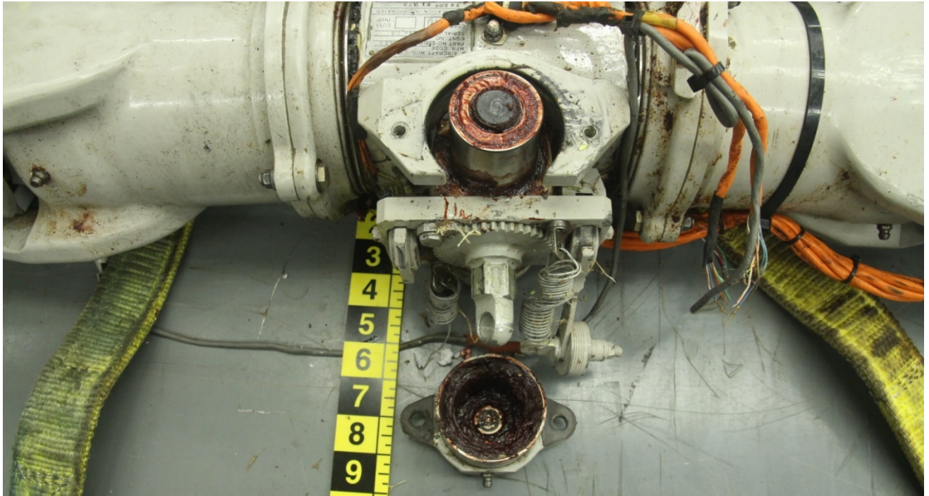
Figure 32 – View of Figure 31, after the bearing cover on this side was removed.
