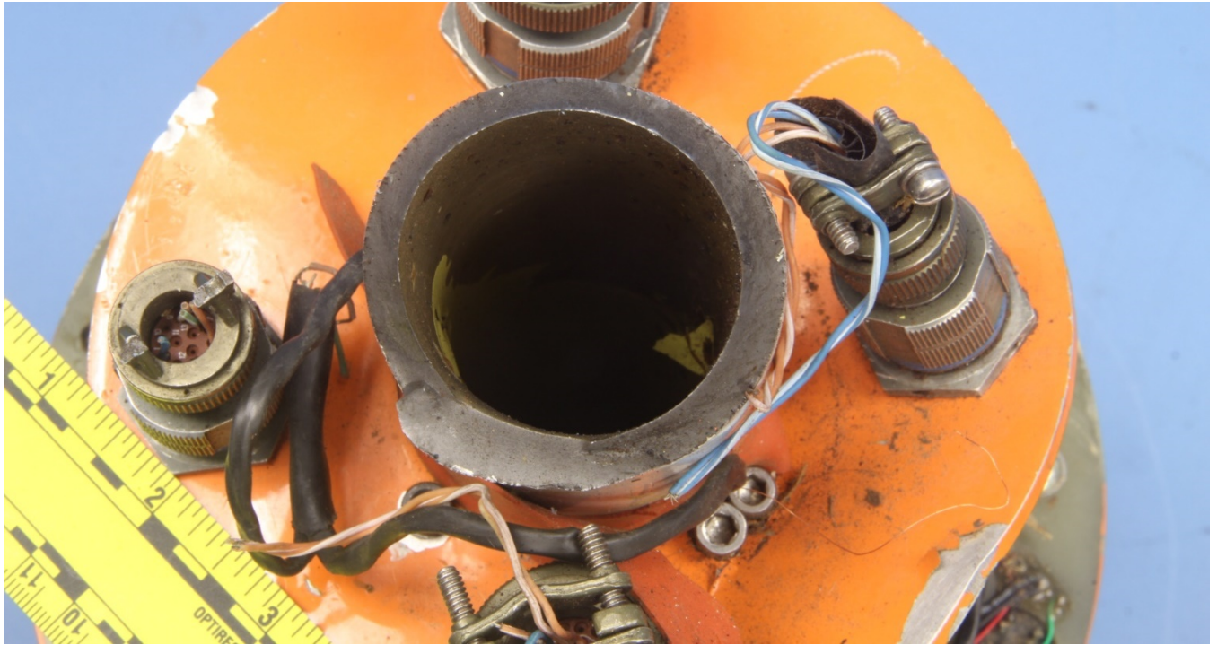
Figure 24 – The lower mast fracture surface viewed facing the reader.
