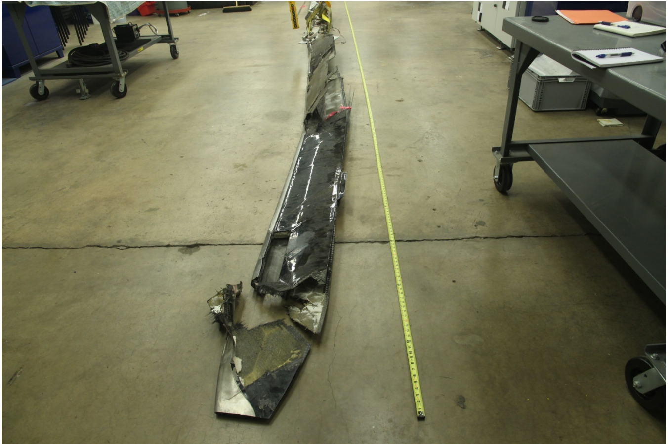
Figure 2 – One section of the main rotor blade fragments laid out in positions consistent with their positions prior to fracture. This is viewed from the tip of Blade B, the blade without instrumentation.
