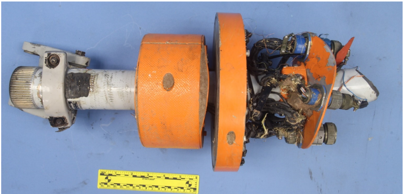
Figure 25 – View of the lower fragment of the main rotor mast (with orange instrumentation affixed). The fracture surface is to the right.
