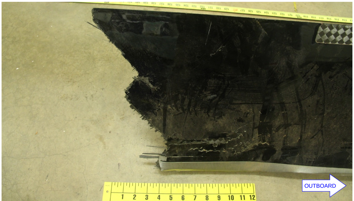
Figure 19 – Mating fracture surface of Blade B from Figure 18.
