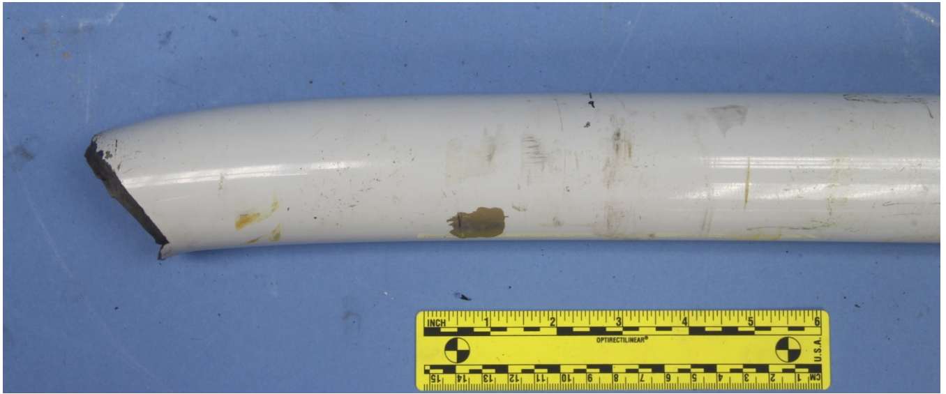
Figure 26 – Side view of the lower mast fracture, after removal of the orange instrumentation.
