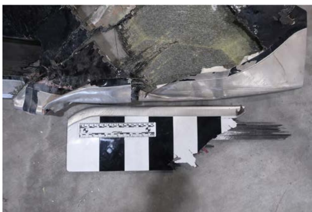
Photo 4: Tail rotor blade leading edge aligned next to main rotor blade tip.
