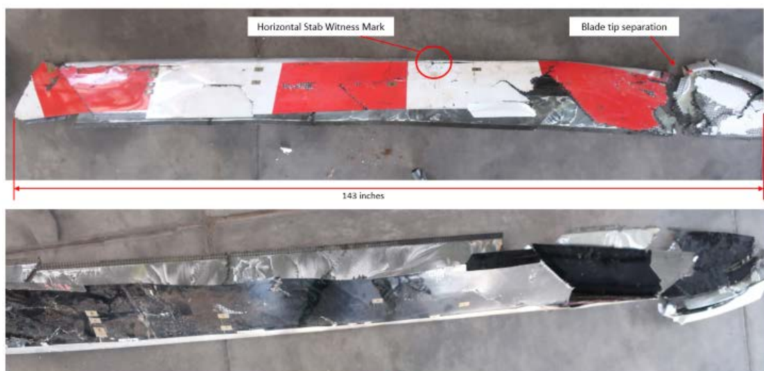
Photo 1: Upper and lower surfaces annotating the horizontal stabilizer spar witness mark and blade tip separation
