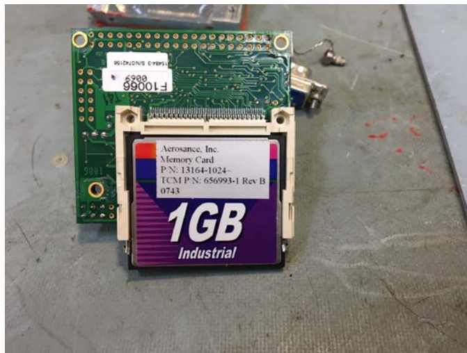
Figure 2. Photo of undamaged CF card inside the unit.
