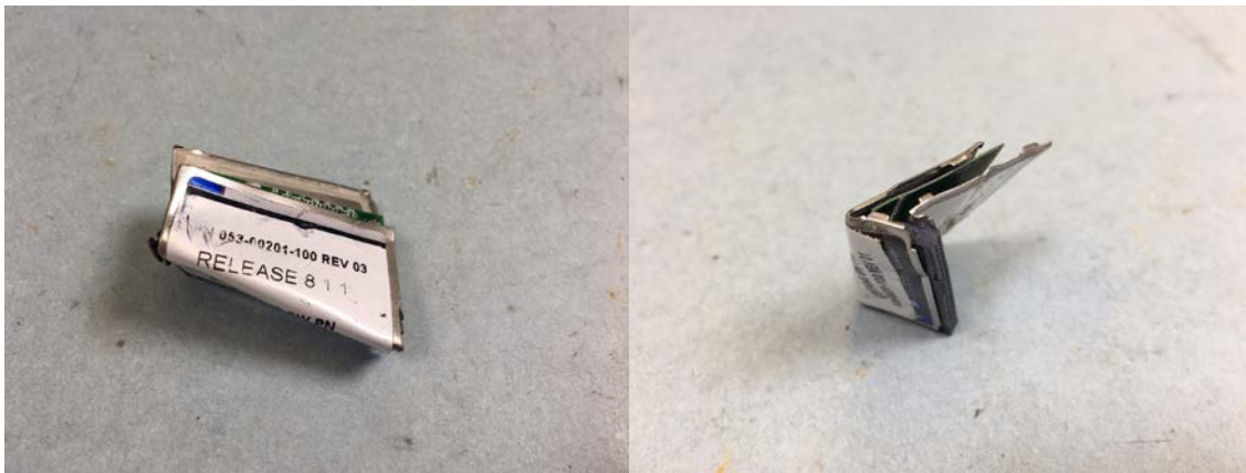
Figure 3. Photos of damaged CF card.
