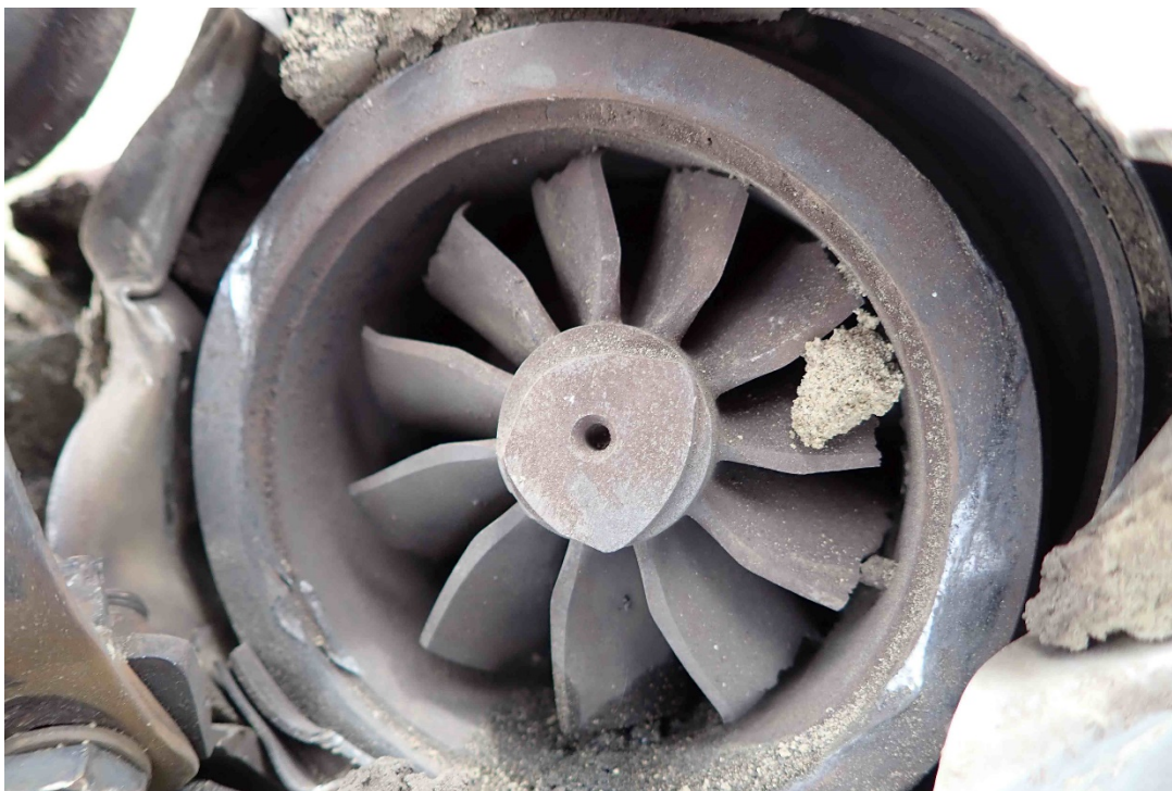
Photo 7 – First turbocharger turbine wheel
