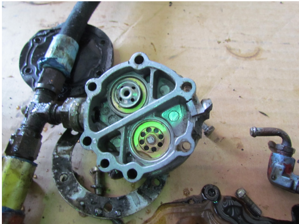
Figure 13: Engine Driven Fuel Pump
