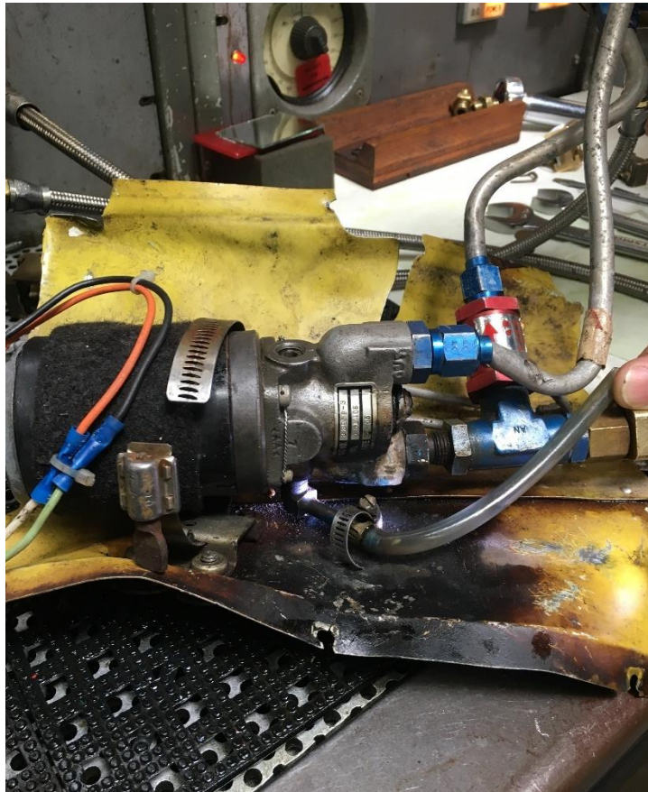
Figure 1: Pressure Test at 14 PSI
