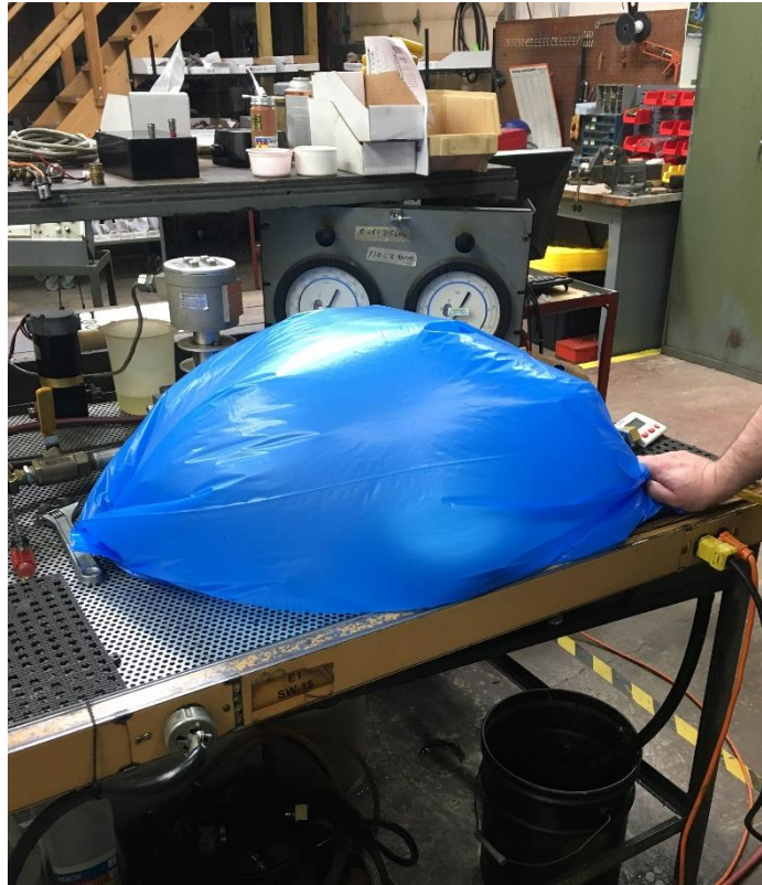
Figure 3: Vacuum pump was attached to the pump outlet and the assembly was placed in a bag.
