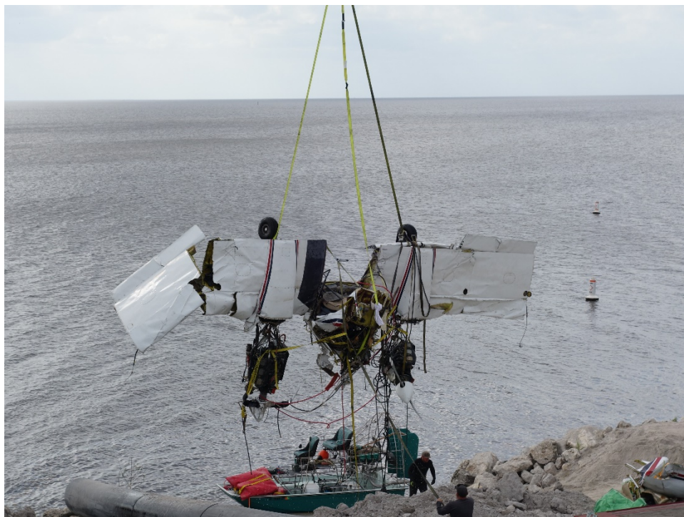
Figure 3: Wings, Engines, and Instrument panel being recovered
