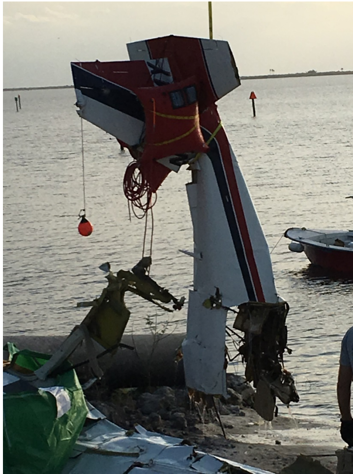
Figure 6: Cabin, Aft Fuselage, and Empennage
