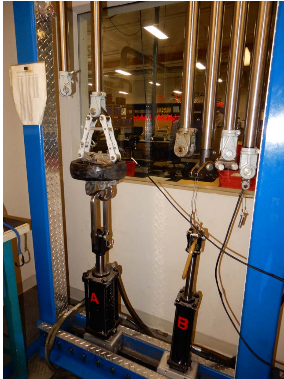
Photo 5 - N64RA cargo hook on test stand.
