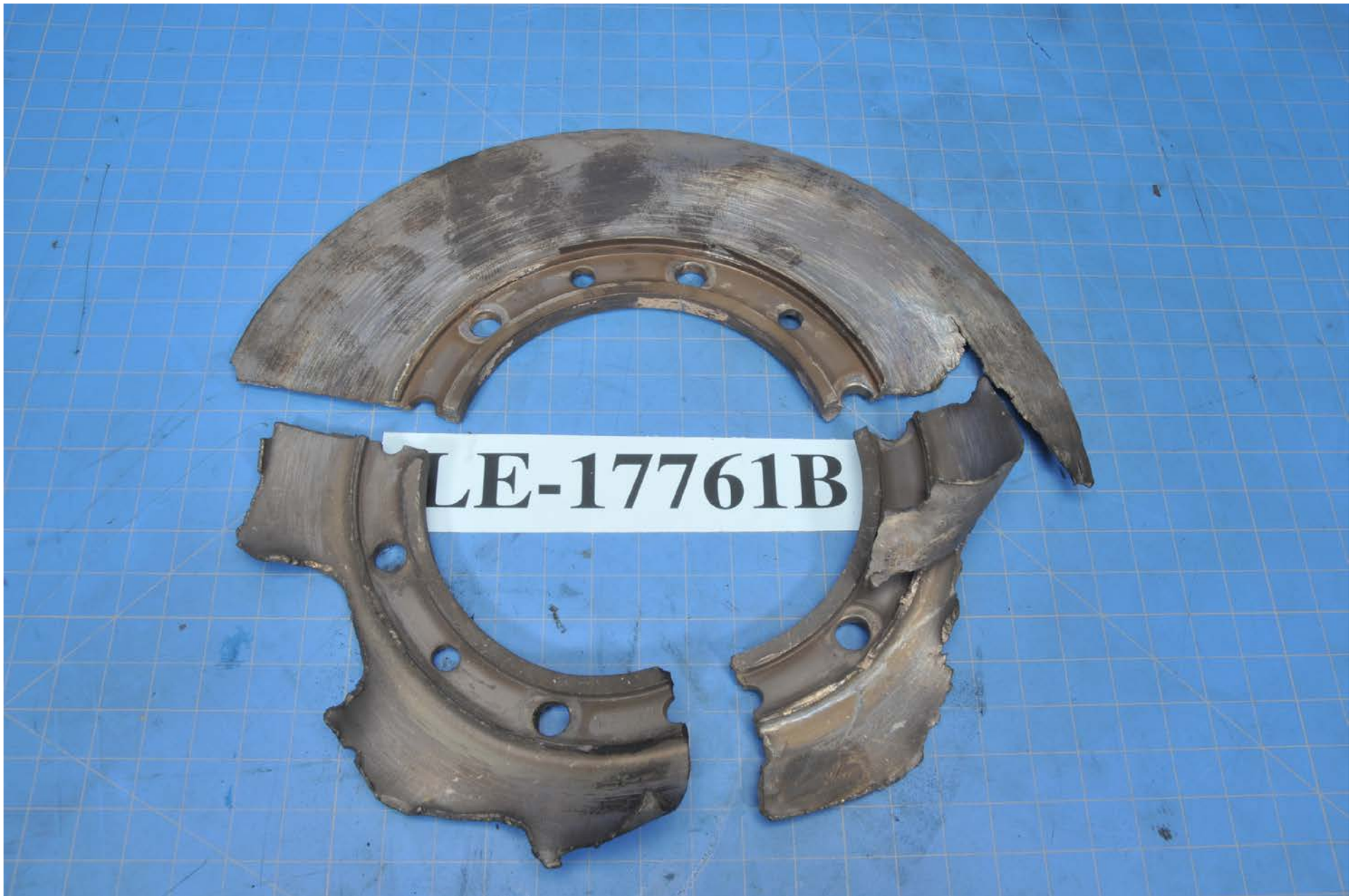
Photo 12 – First stage sealing disk shown in three fragments. Photo curtesy of Honeywell Aerospace.
