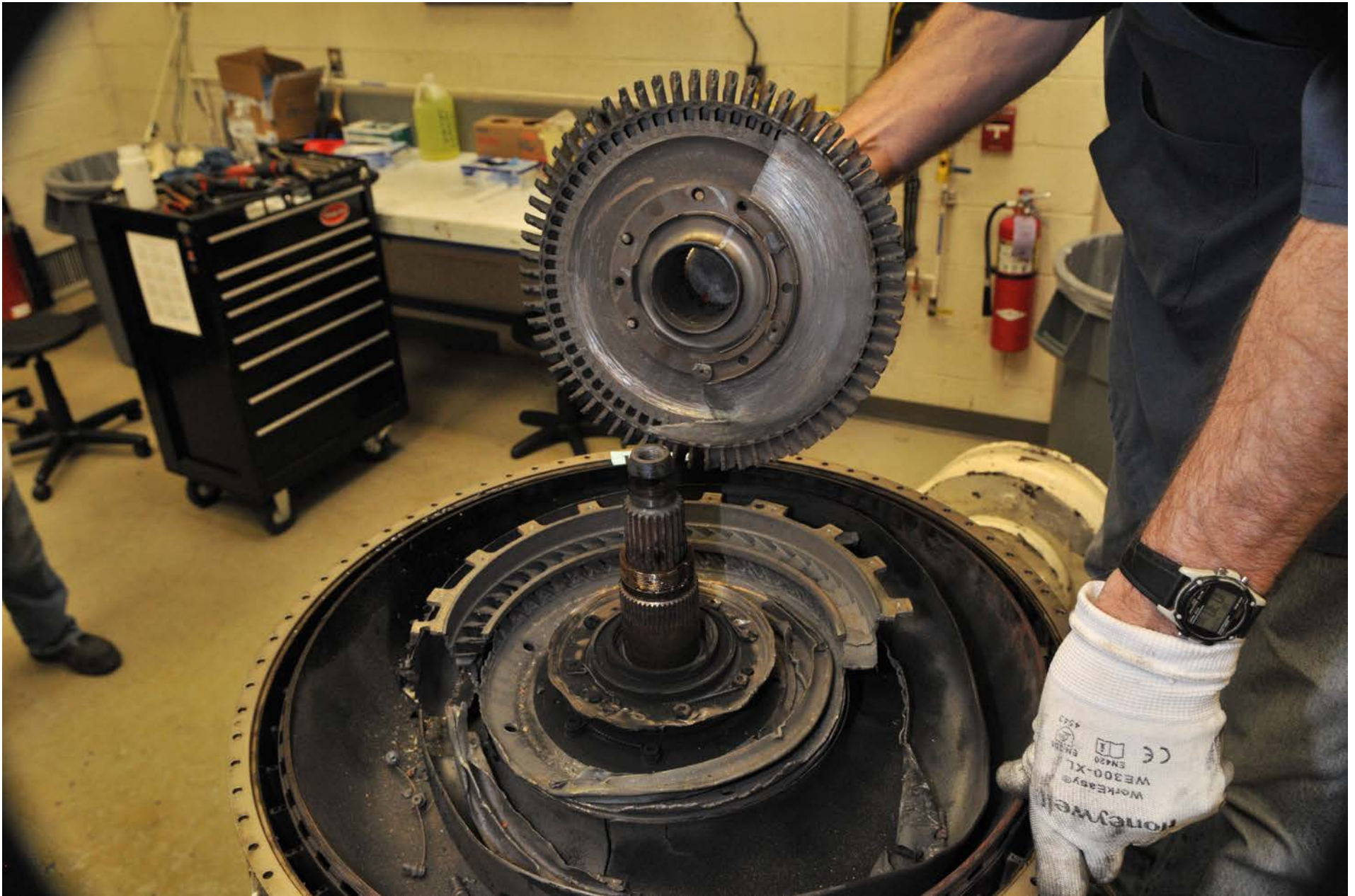
Photo 11 – First-stage turbine rotor with a portion of the first stage sealing disk remaining attached.
