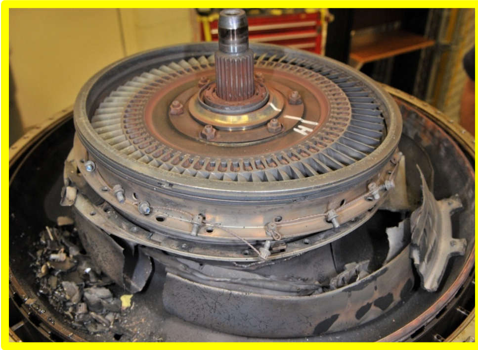
Photo 3: T-53-L-13B Engine showing the gas producer turbine rotor assembly and internal engine damage.
