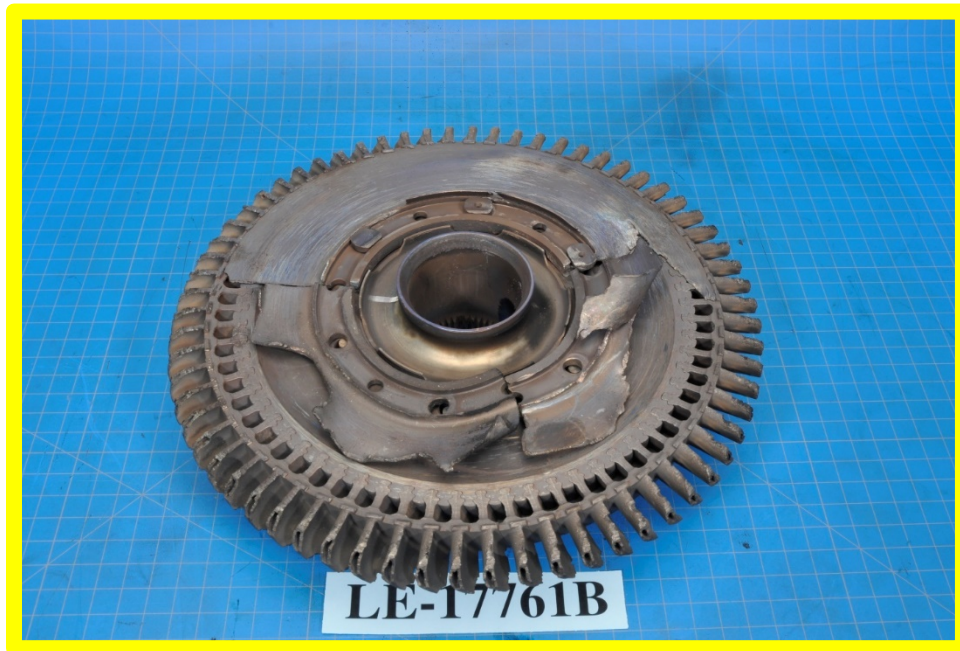
Photo 5: First stage gas producer turbine rotor with sealing disk resting in place. Photo courtesy of Honeywell Aerospace.
