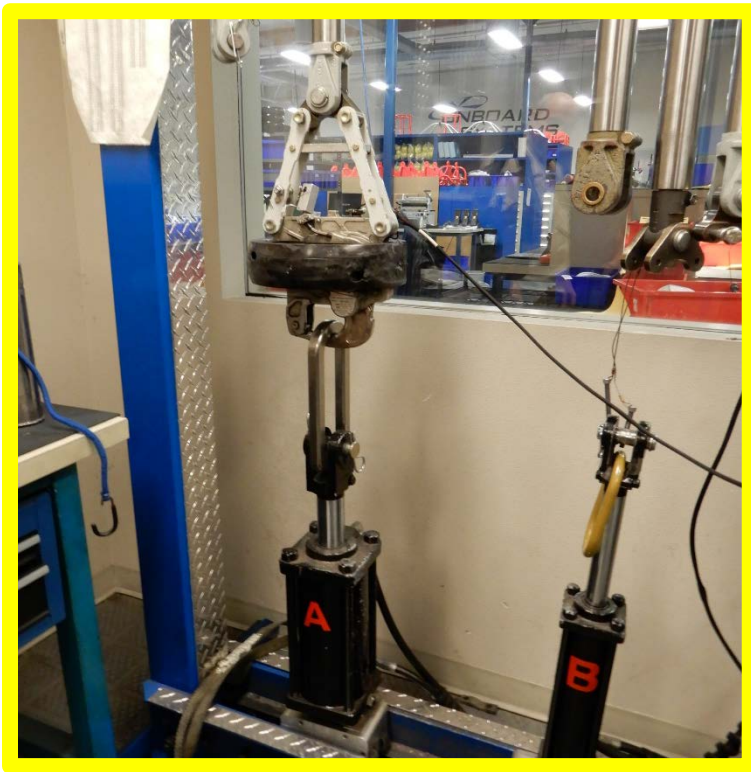
Photo 9. Cargo hook examination, showing cargo hook on test stand.
