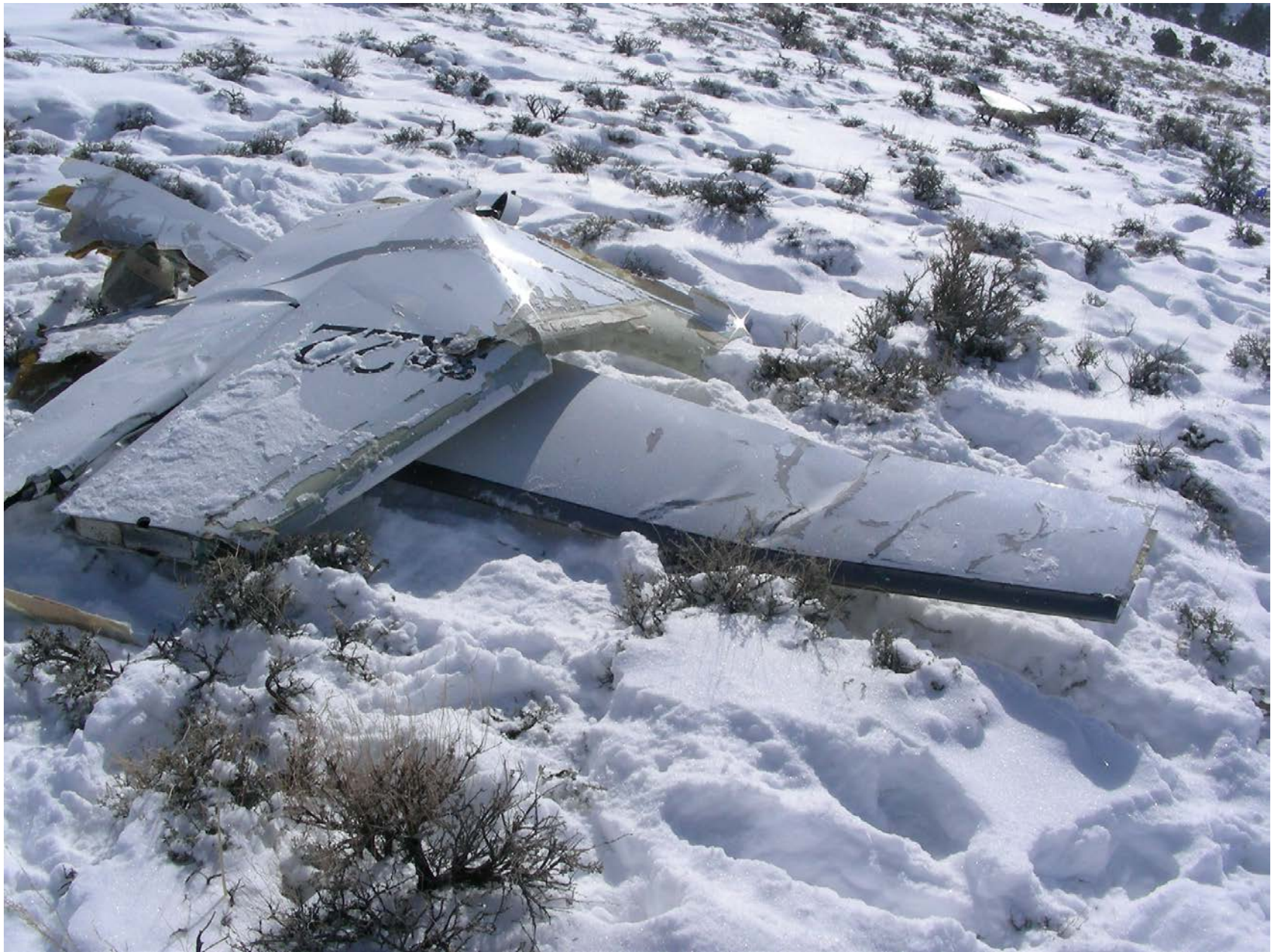
Photo 5 – view of empennage – horizontal and vertical stabilizers and rudder
