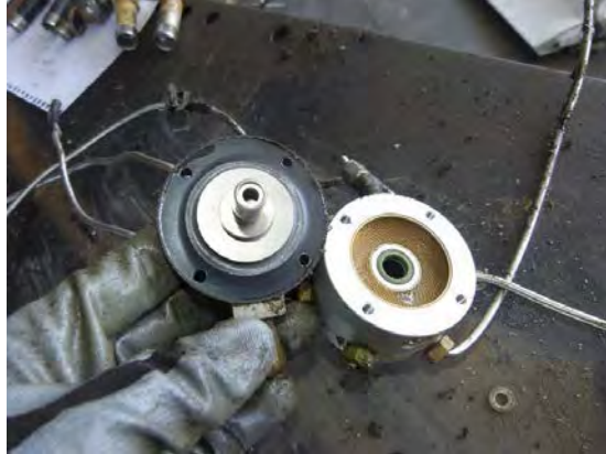
Figure 12 - fuel manifold valve
