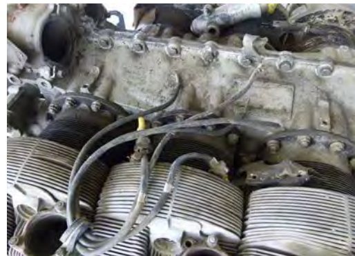
Figure 8 - ignition harness leads
