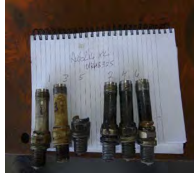
Figure 10 - bottom spark plugs
