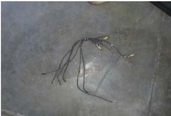
Figure 7 - ignition harness leads
