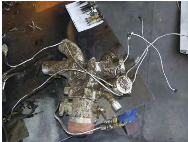
Figure 2 - photo of induction system
