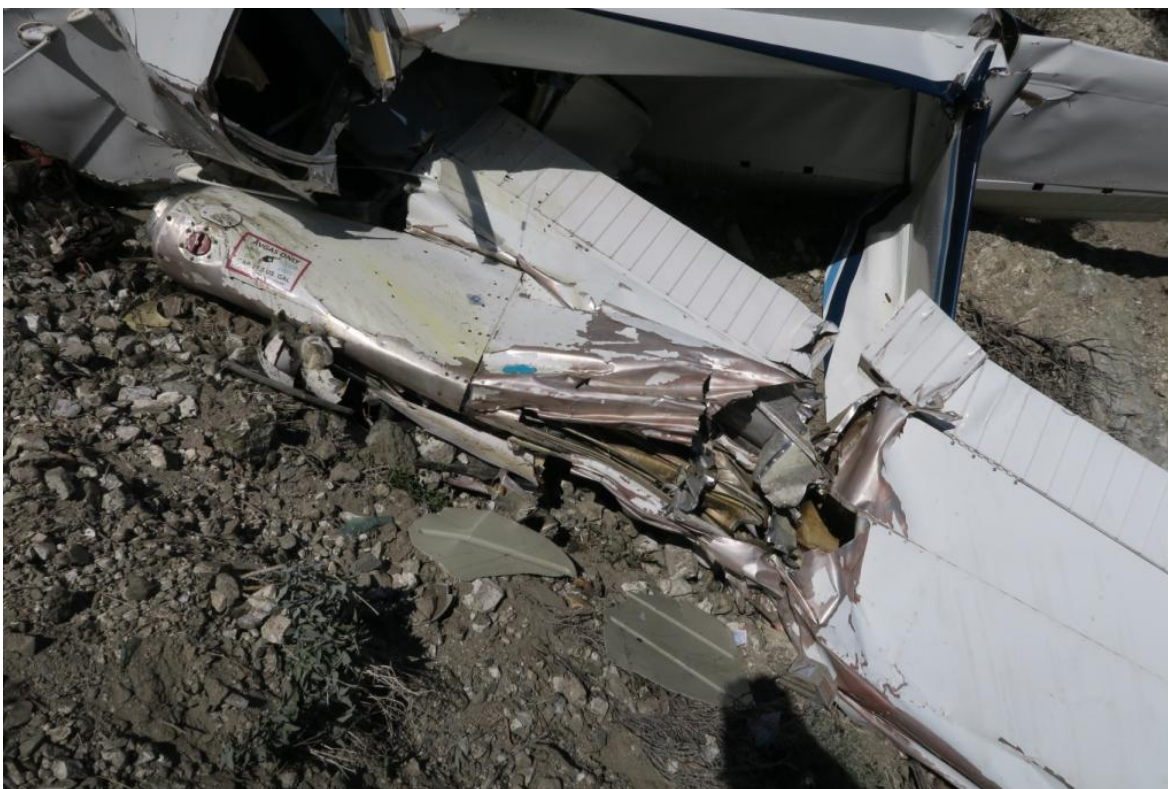
Figure 15 - Left Wing LE Crush Damage
