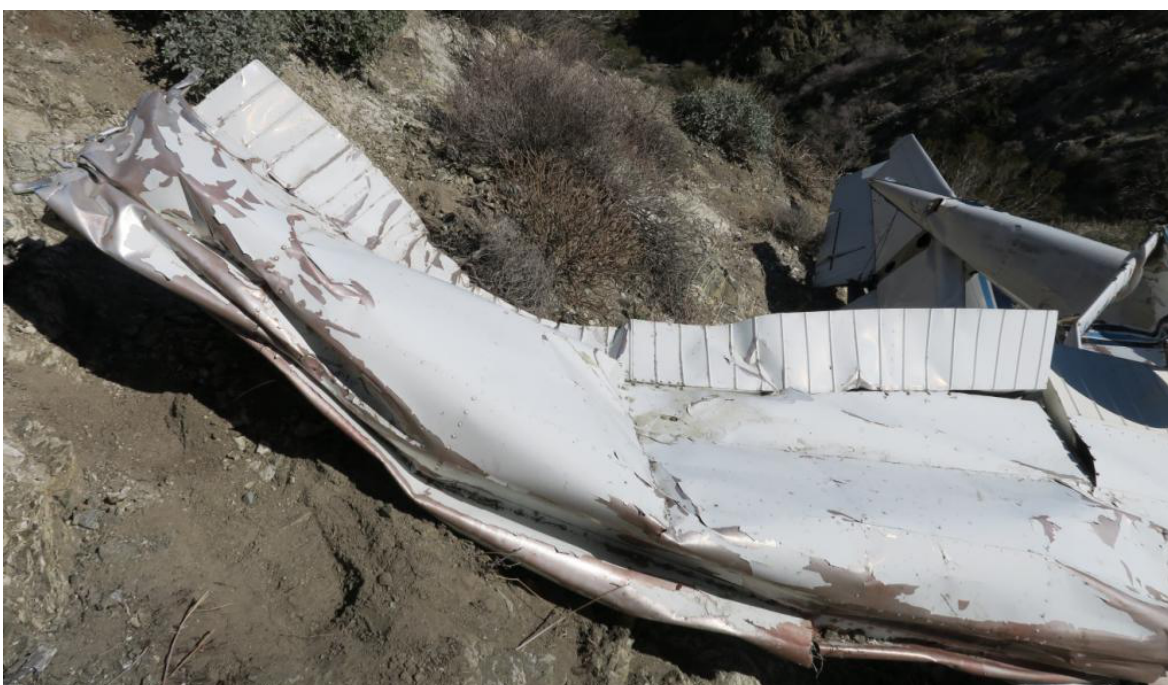
Figure 16 - Right Wing LE Crush Damage
