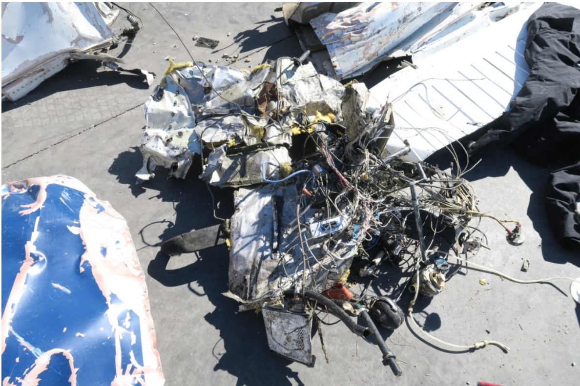
Figure 4 - Cockpit Avionics & Wiring
