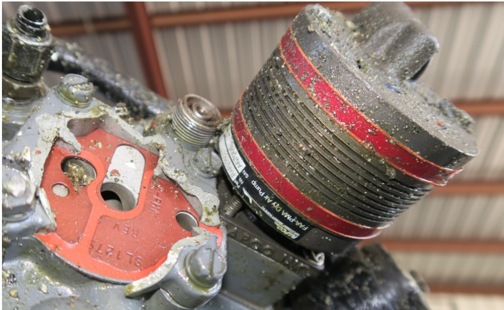
Figure 28 - Vacuum Pump (in situ)
