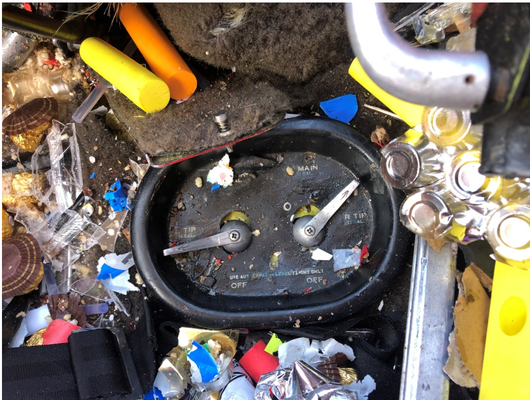
Figure 4: View of the fuel selector valve handles.
