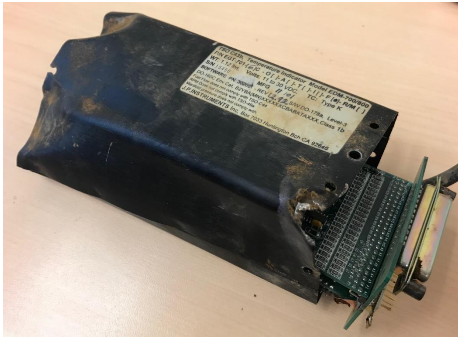
Figure 1. Damaged exterior of EDM.
