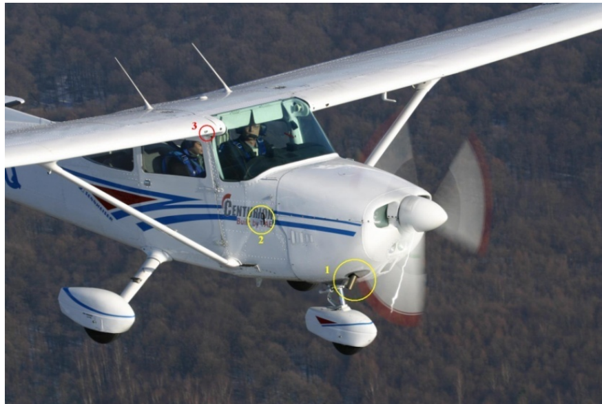
Figure C-10. Cessna 172 Locations for the Exhaust Tailpipe (1) and Fresh Air Inlets (2 and 3) [C-18]
