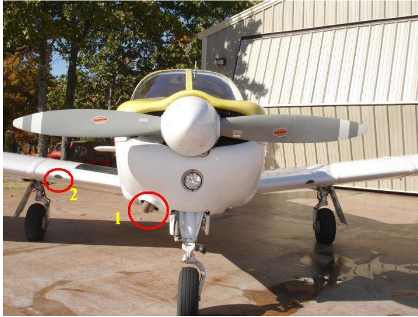
Figure C-11. Piper PA-28 Locations for the Exhaust Tailpipe (1) and Fresh Air Inlet (2) [C-19]
