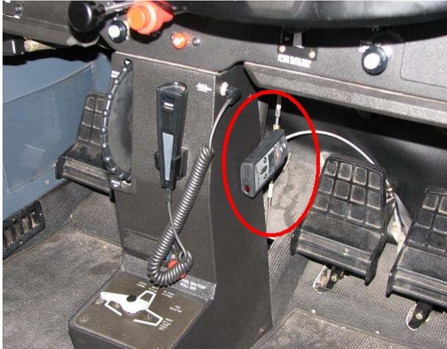
Figure B-1. Carbon Monoxide Detector Attached to the Instrument Panel With a Belt Clip
