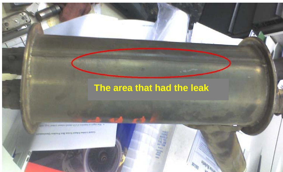
Figure D-7. The Muffler That had the Leak but was not Detected by Visual Check
