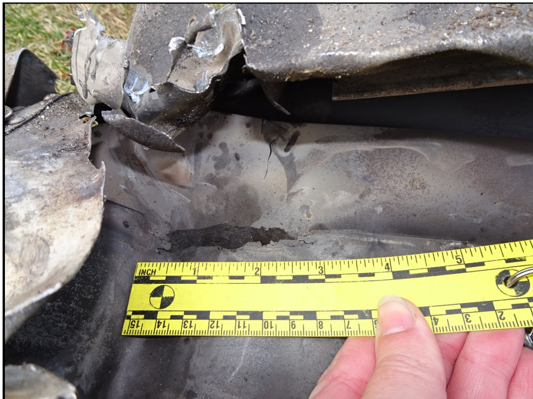
Photo 10 – Aft Exhaust Muffler
