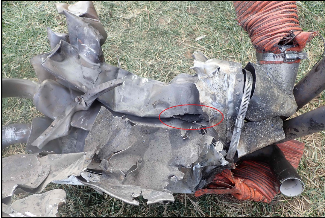
Photo 9 – Exhaust Muffler System with Hole Circled
