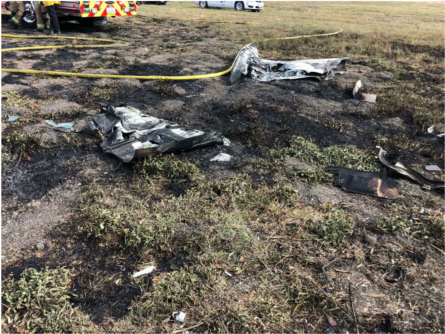
Photo 6 – View of portions of cowling and left wing tip.
