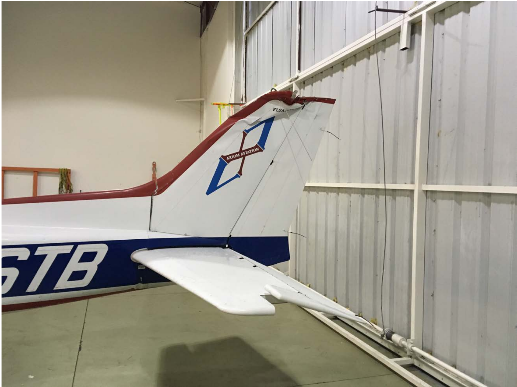
Photo 3 – Damage to the Empennage
