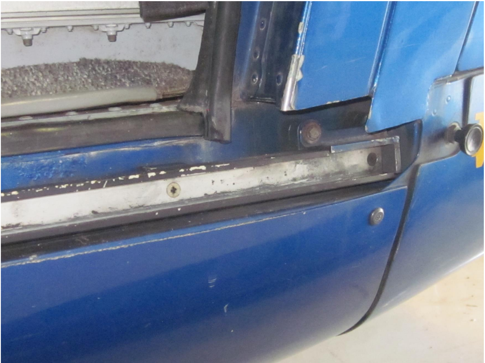
Photo 4 – Left Side Sliding Door Lower Track
