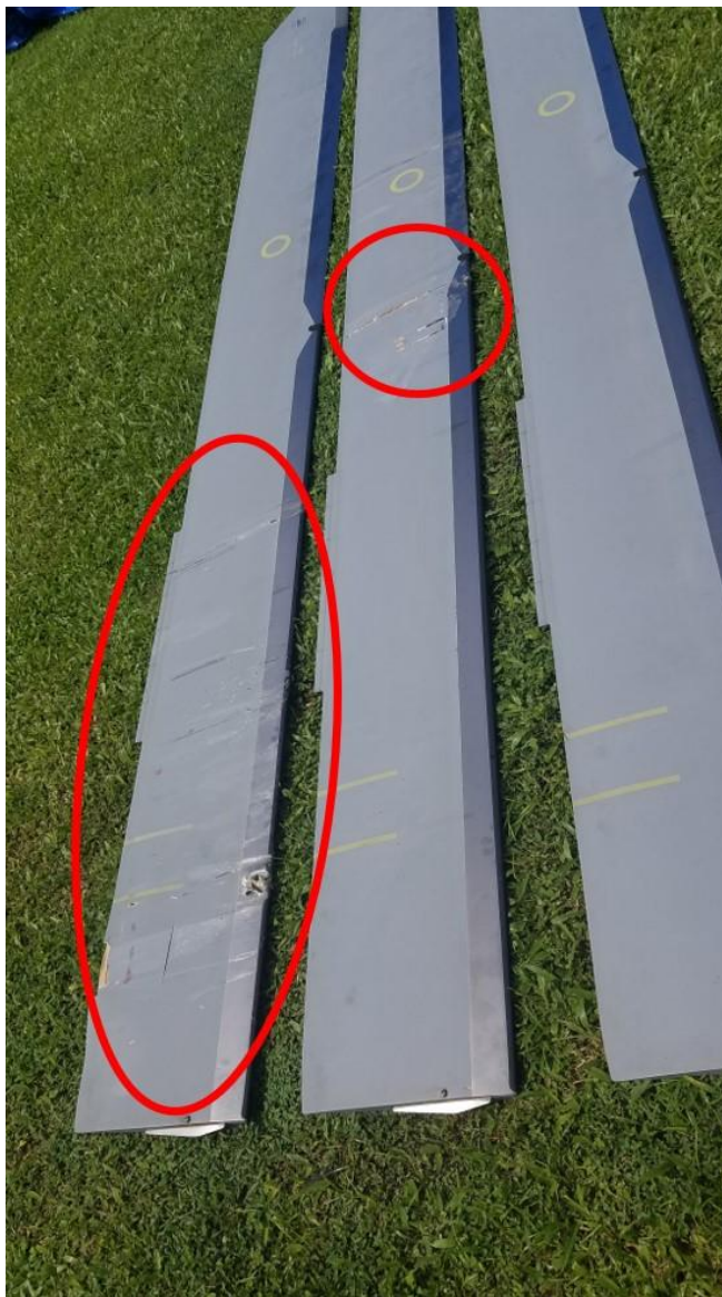
Photo 6 -Main Rotor Blades Showing Damage circled in Red
