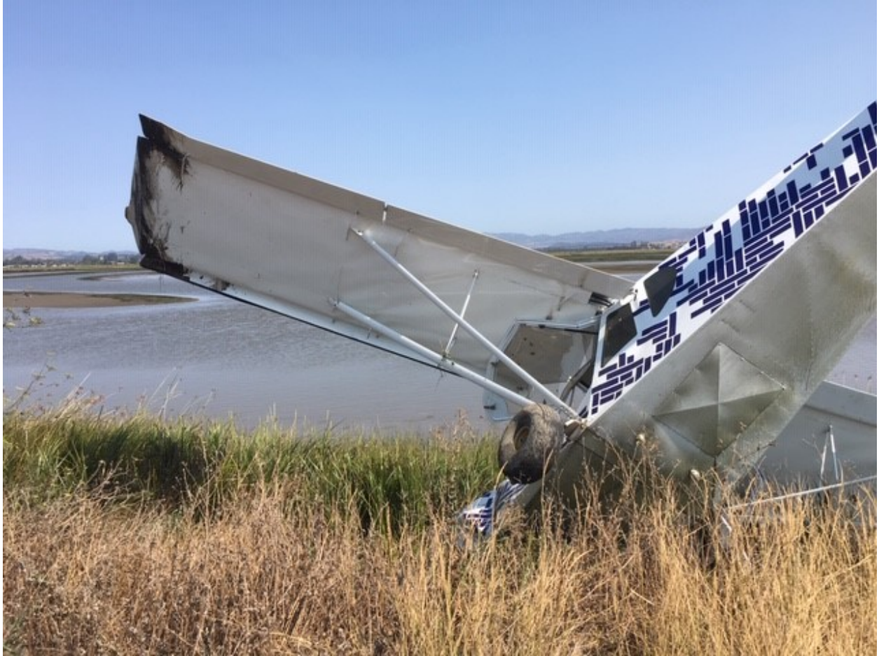
Figure 5 - Left Wing Damage
