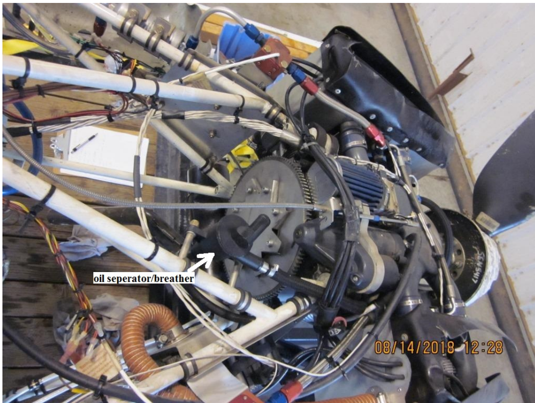
Figure 7 - Engine w Oil Separator Highlighted
