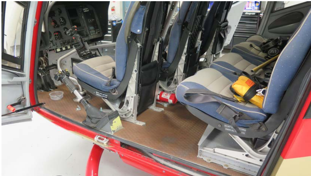
Photo 17. Stowage location of fire extinguisher on Papillon's EC130 B4.
