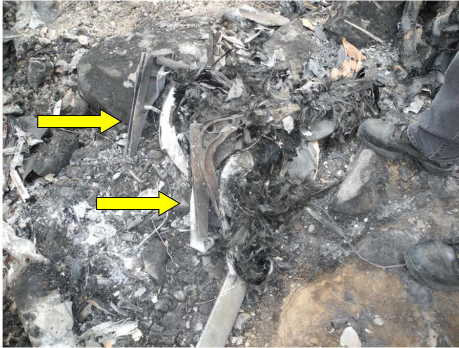
Photo 8. Thermally damaged seat found immediately to the front right of the helicopter (left and right frames visible).
