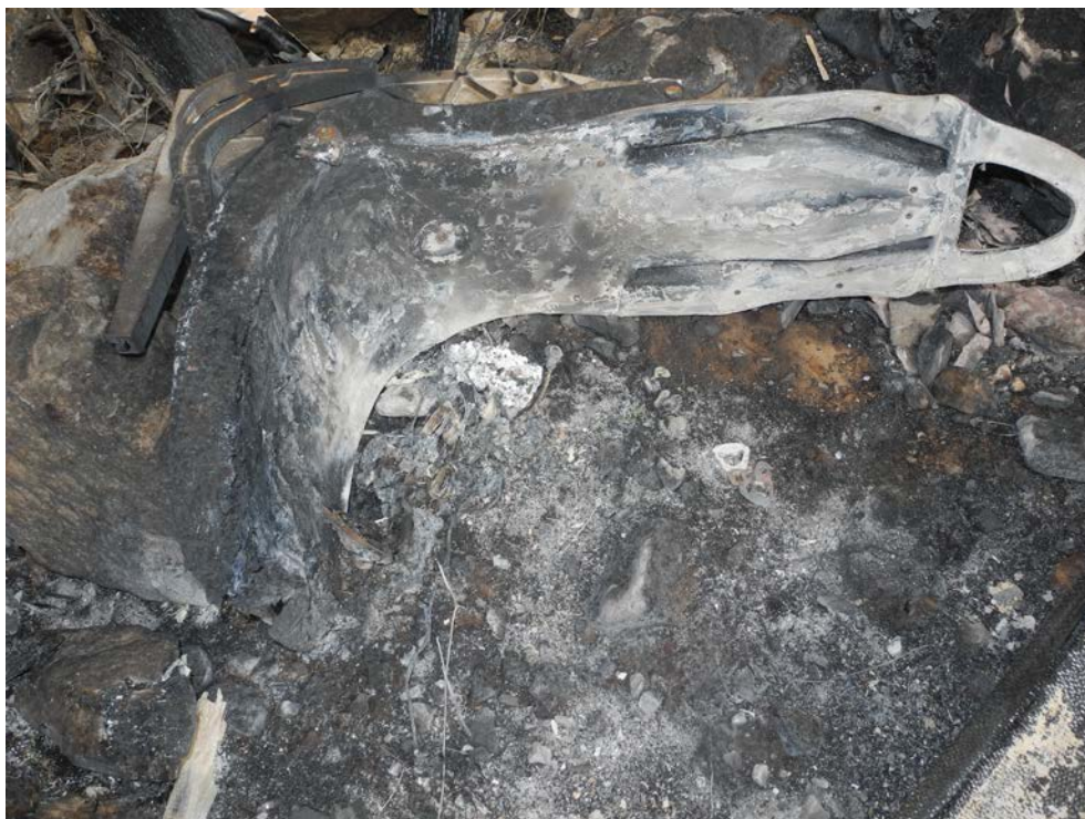
Photo 6. Close-up of the thermally damaged seat found near a small tree.
