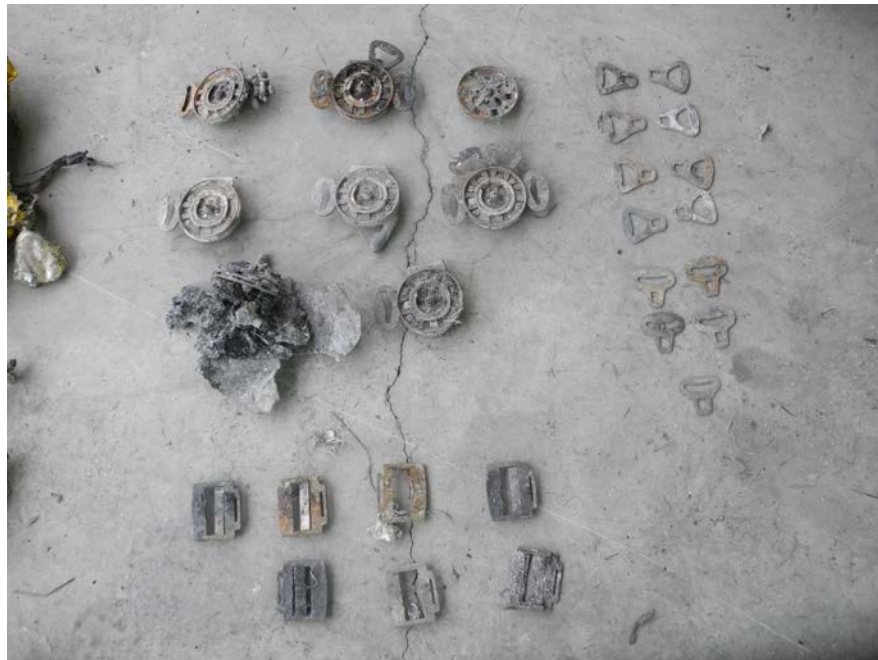
Photo 15. Rotary seatbelt buckles, insert tabs, and adjusters identified in the wreckage.
