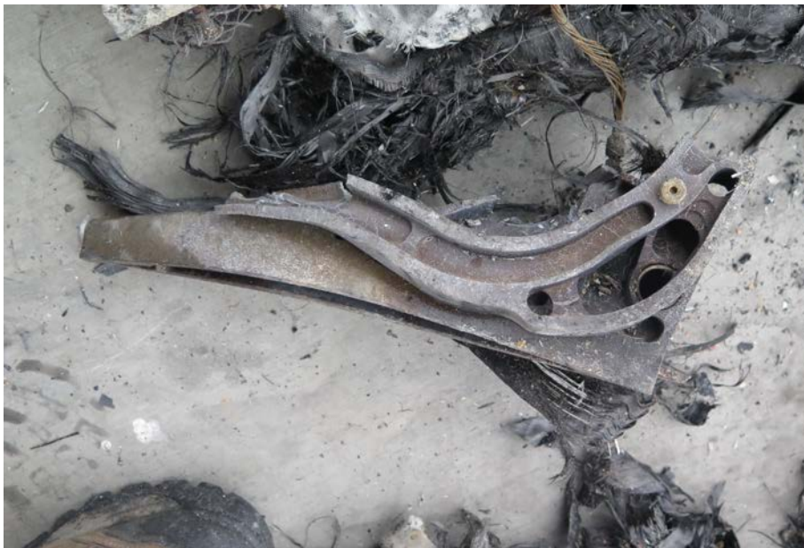
Photo 9. Left frame of seat found immediately to front right of helicopter (front web was fractured; aft web was partially fractured).
