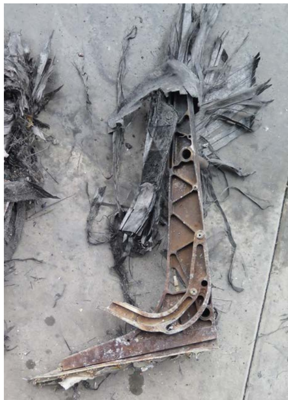
Photo 12. Left frame of aft left seat.
