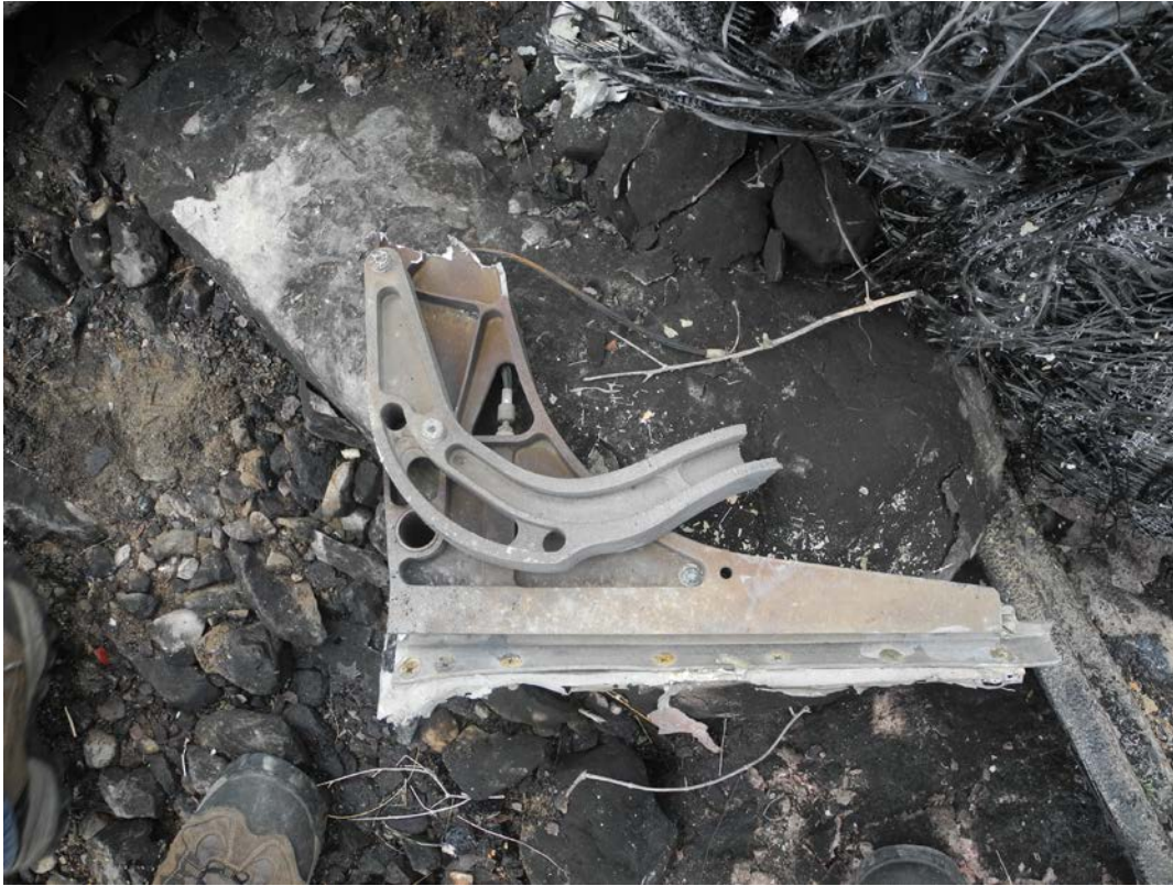
Photo 13. Right frame of aft left seat.
