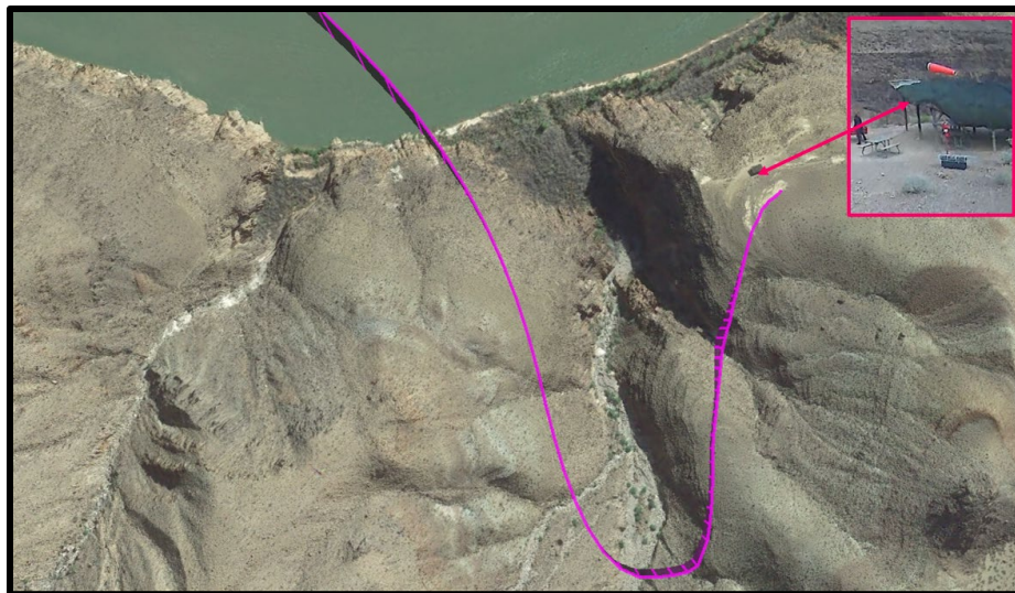
Figure 11: Track of Helicopter 23 Landing Showing Windssock Just Prior to Touchdown
