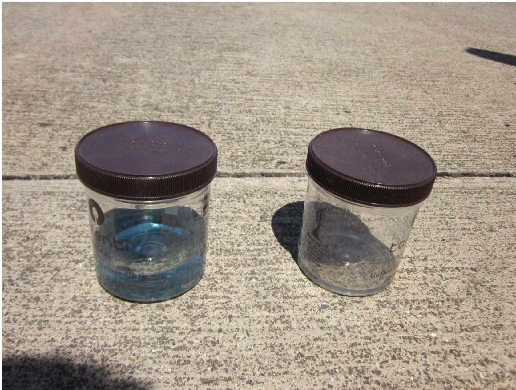
Photo 2. Left – sample from the right tank. Right – fuel collected from the fuel line
