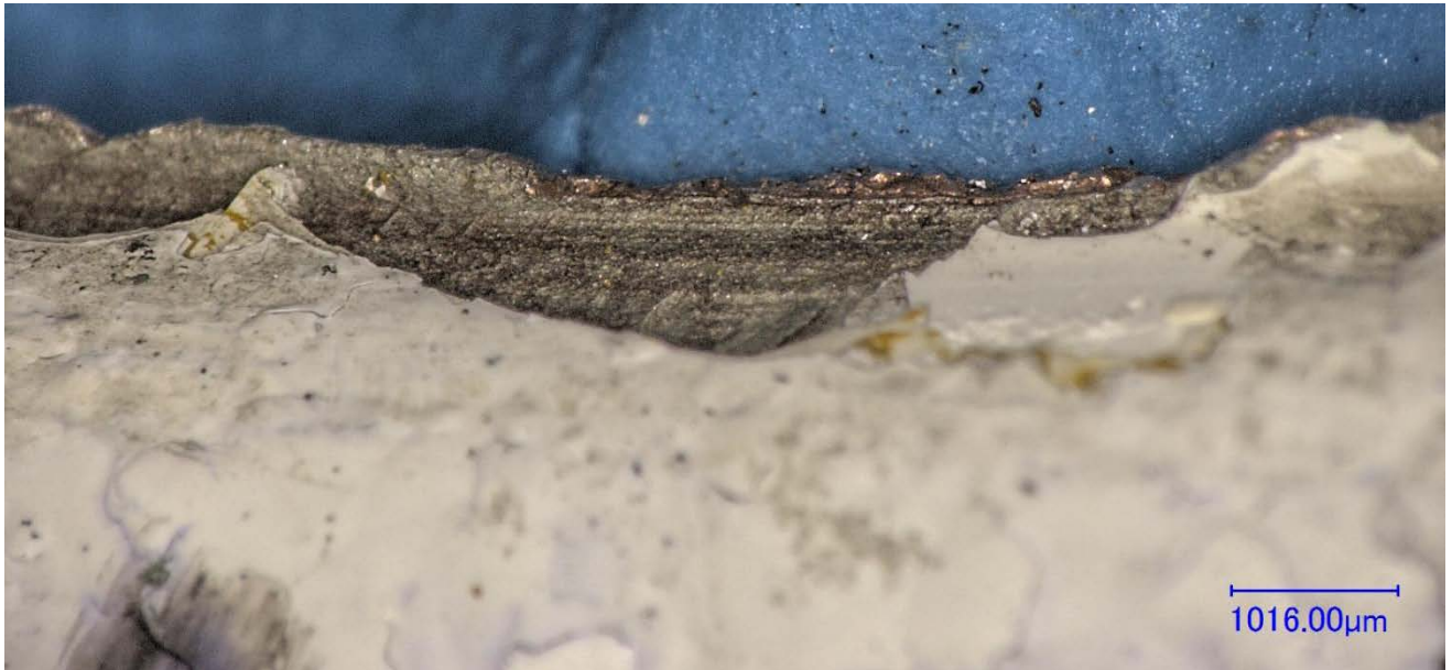
Figure 13 – The outside view of the fracture surface in Figure 12, showing circumferential weld lines parallel to the surface.
