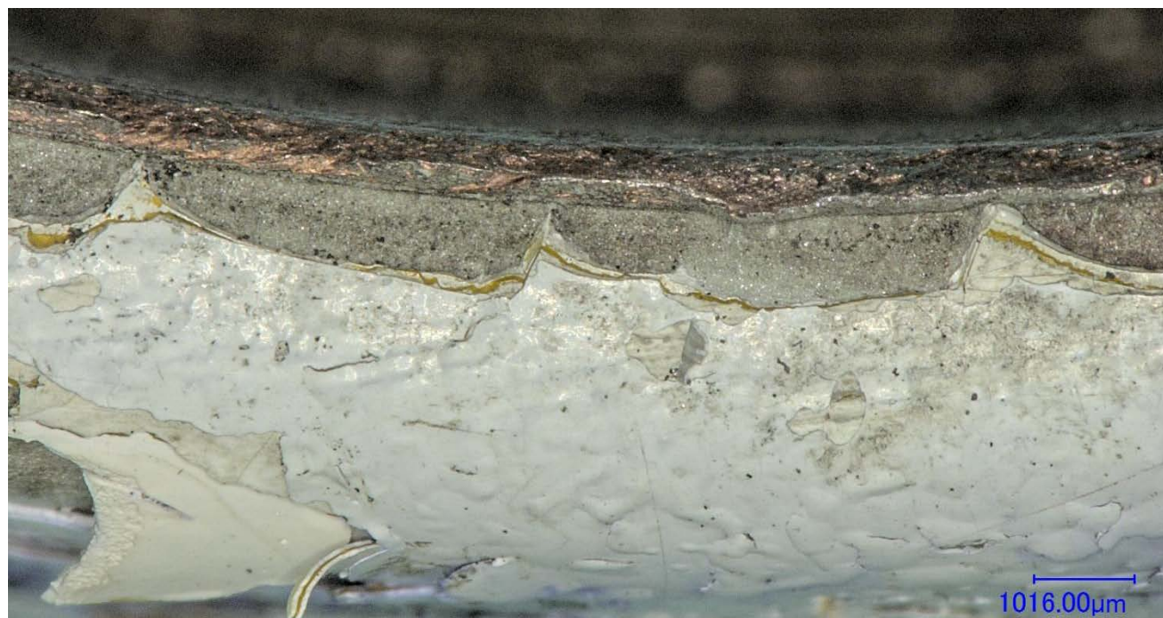
Figure 10 – View of the upward face of the joint fracture surface, showing the smeared bushing material, the fractured white paint and the underlying joint steel material.
