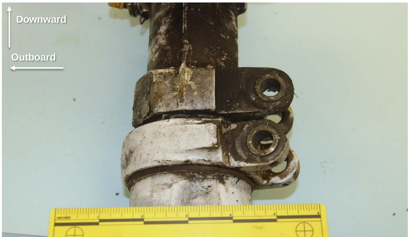
Figure 8 – The loose joint after removal of the linkage and bolt assemblies, viewed forward looking aft.
