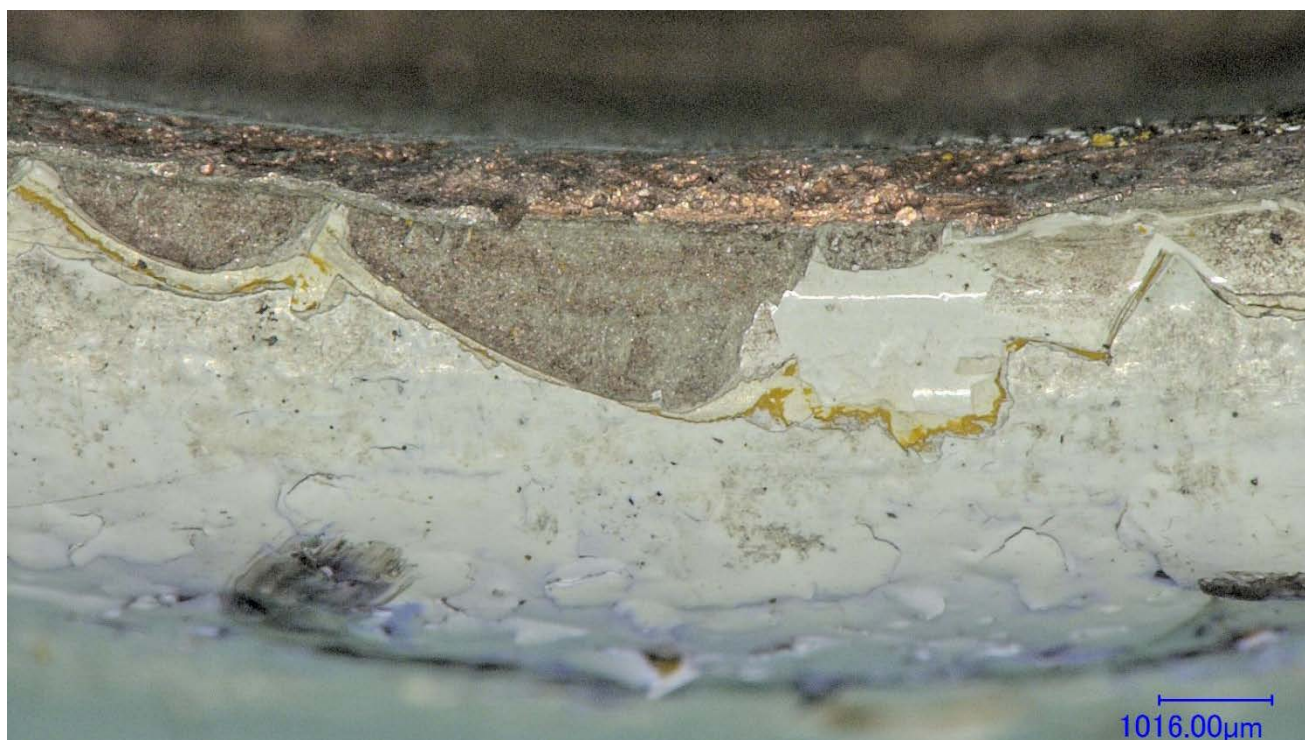
Figure 12 – View of fracture features on the bushing portion of the joint fracture surface.
