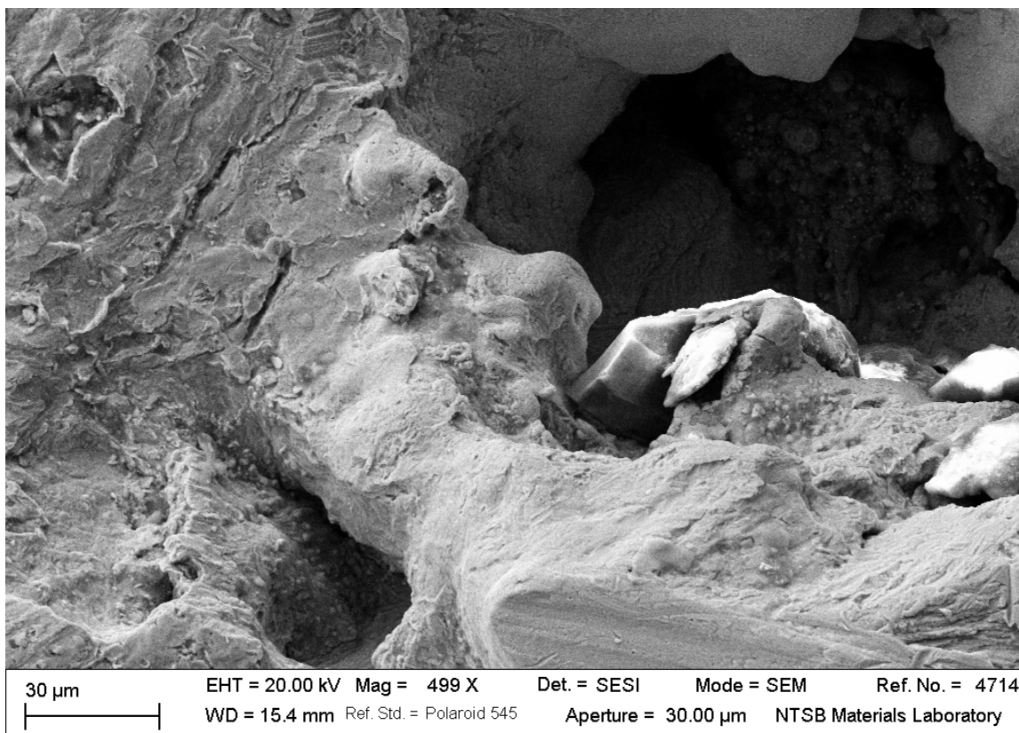
Figure 18 – SE micrograph of a closer view of Figure 17, absent pore cracking.
