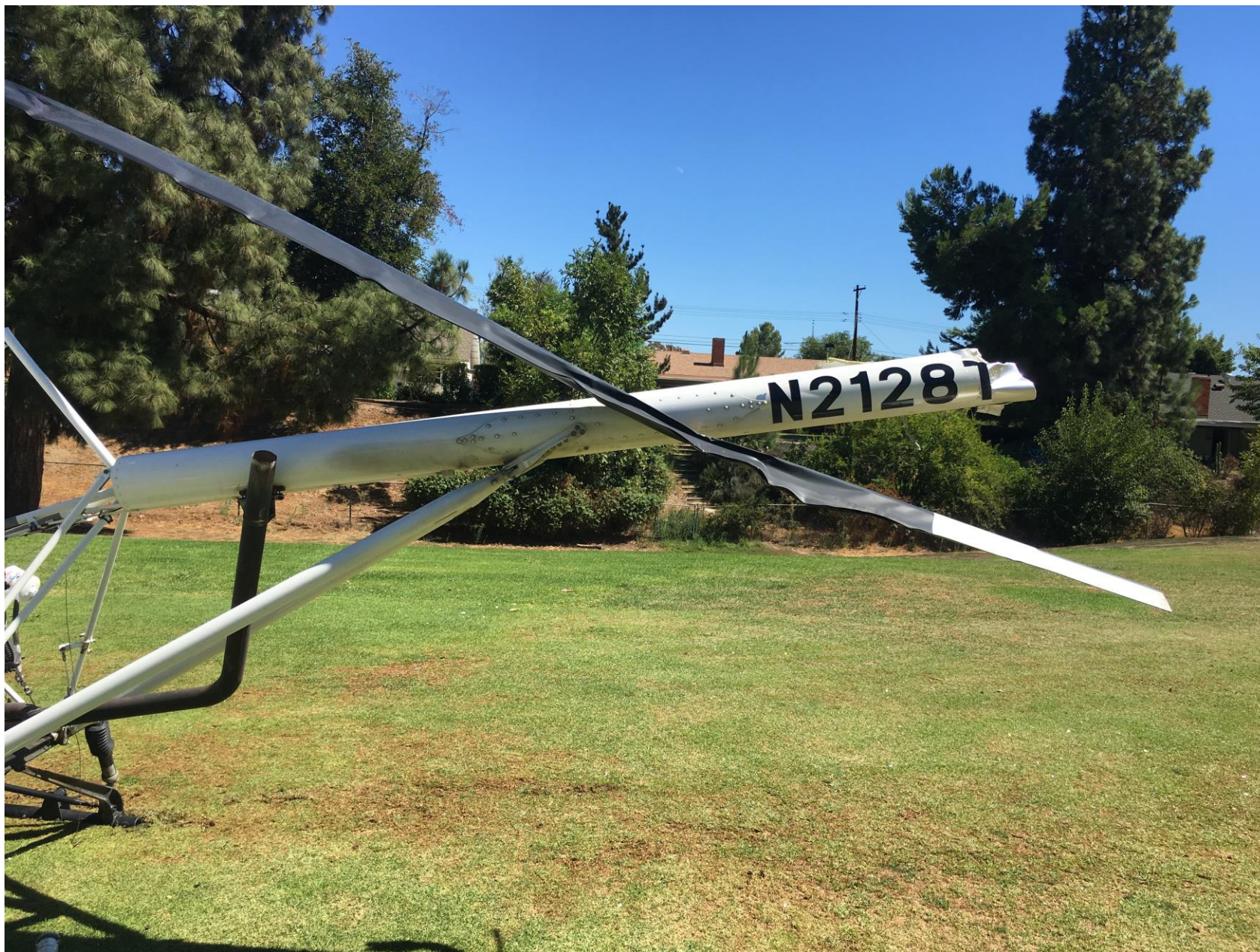
Photo 2 – Accident site, tailboom separation and main rotor blade damage. (Courtesy of the FAA)
