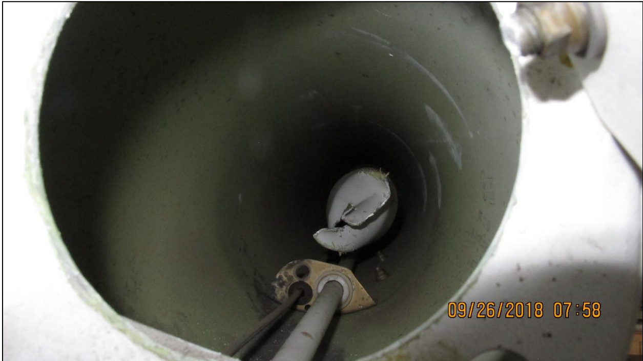
Figure 2-Driveshaft Separation in the Tailboom
