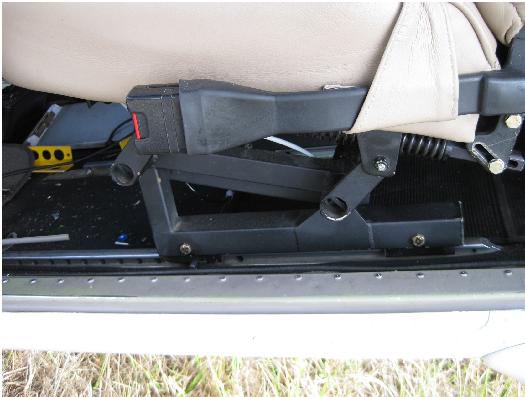
Photo 2 – Seat Rail (Photo Courtesy of the FAA)
