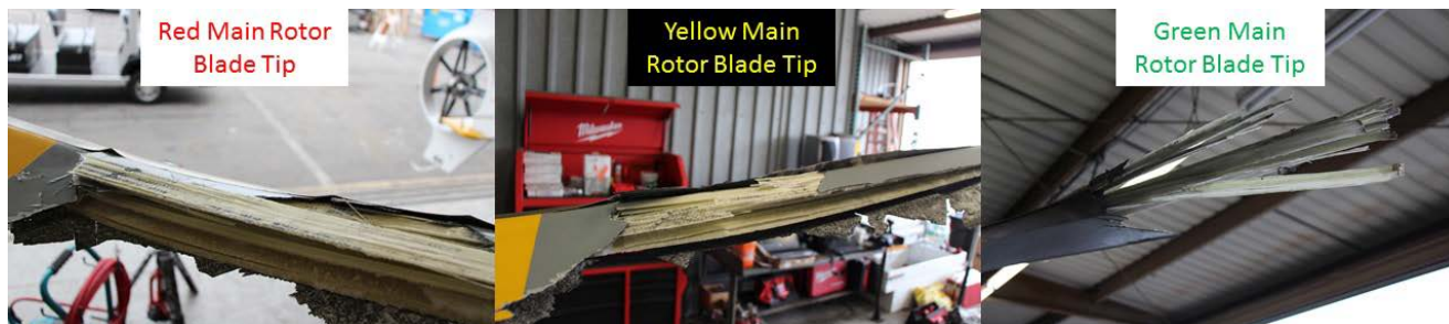
Photograph 2: Main Rotor Blade Tip Damage
