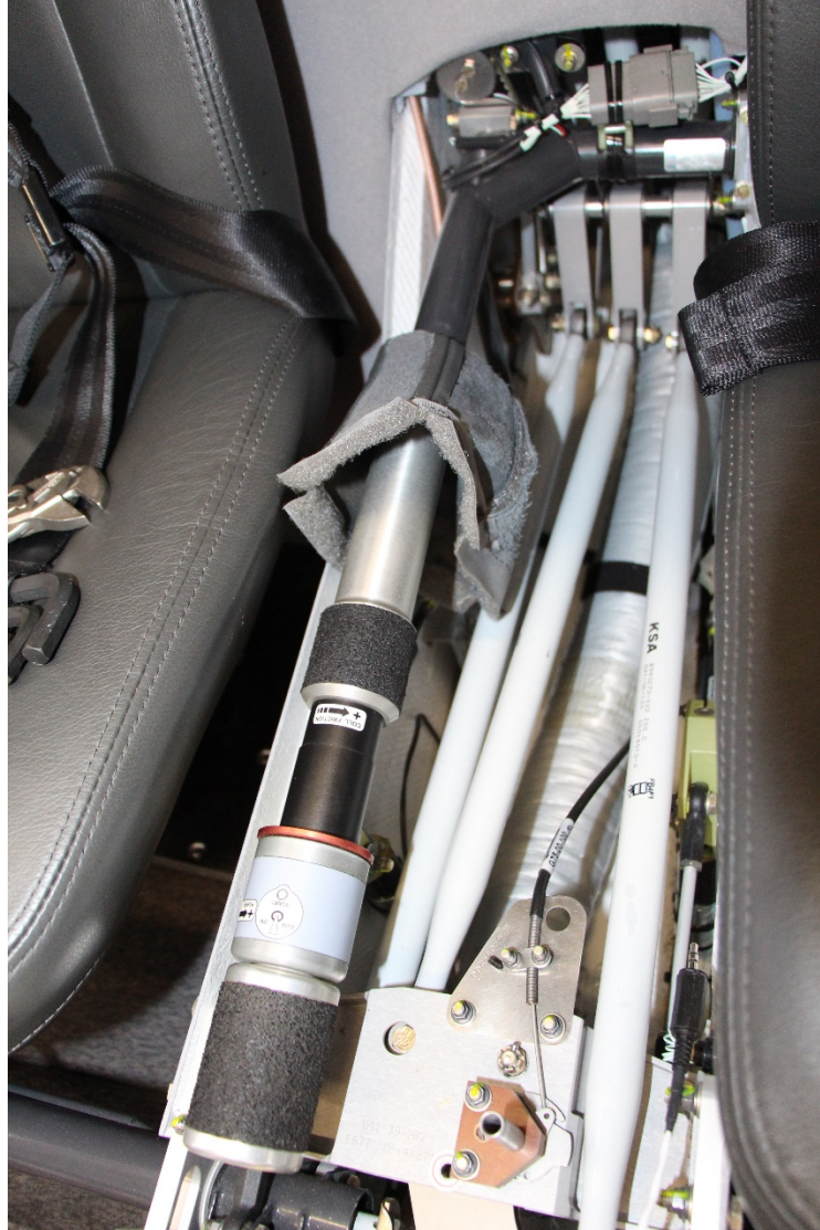
Photograph 3: Center Console without Cover, Right Seat Collective Control, Correlator (top of photo), and Governor Adjustment (top of photo)
