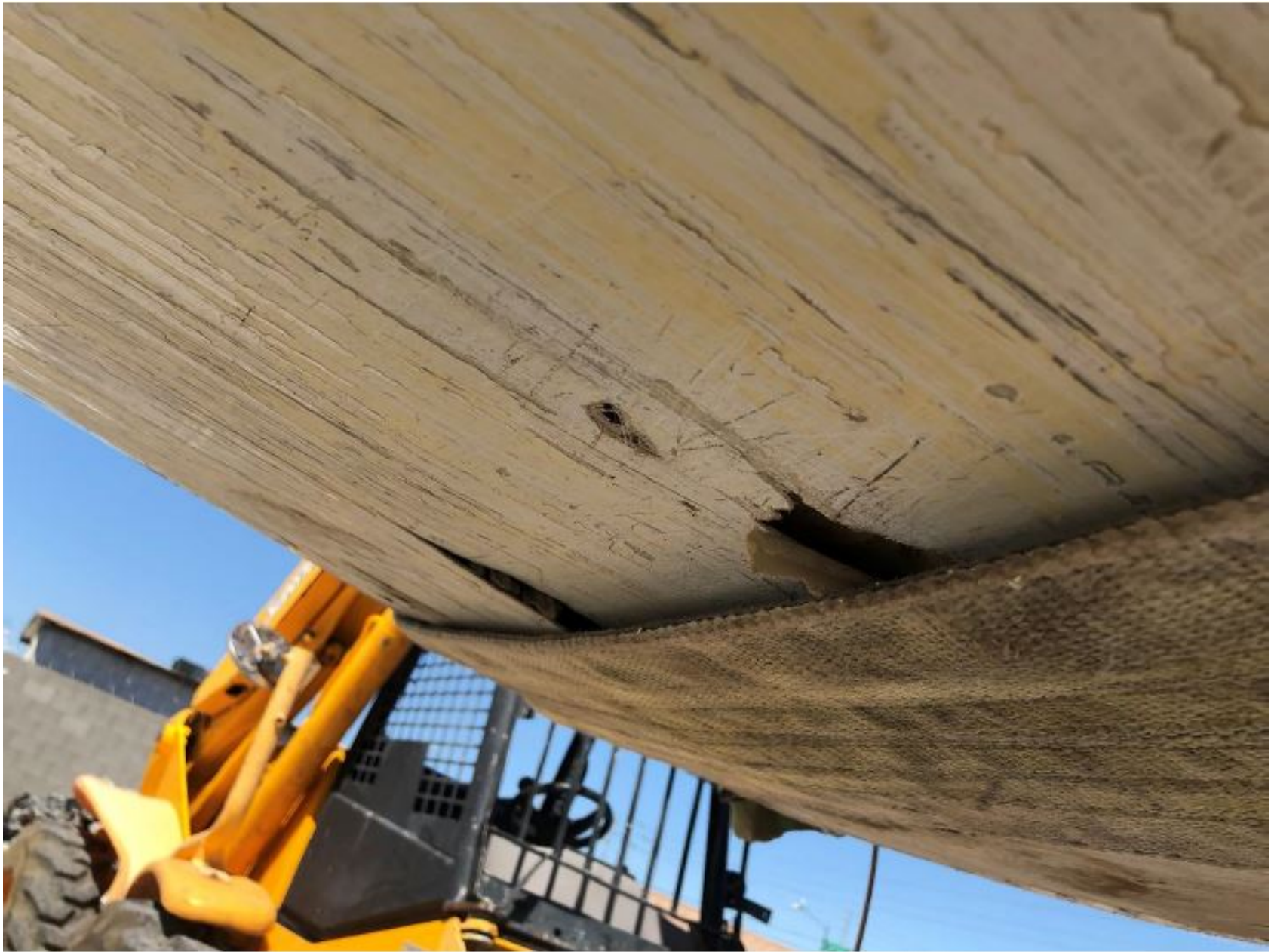
Photo 2 – Damage to Lower Aft Fuselage
