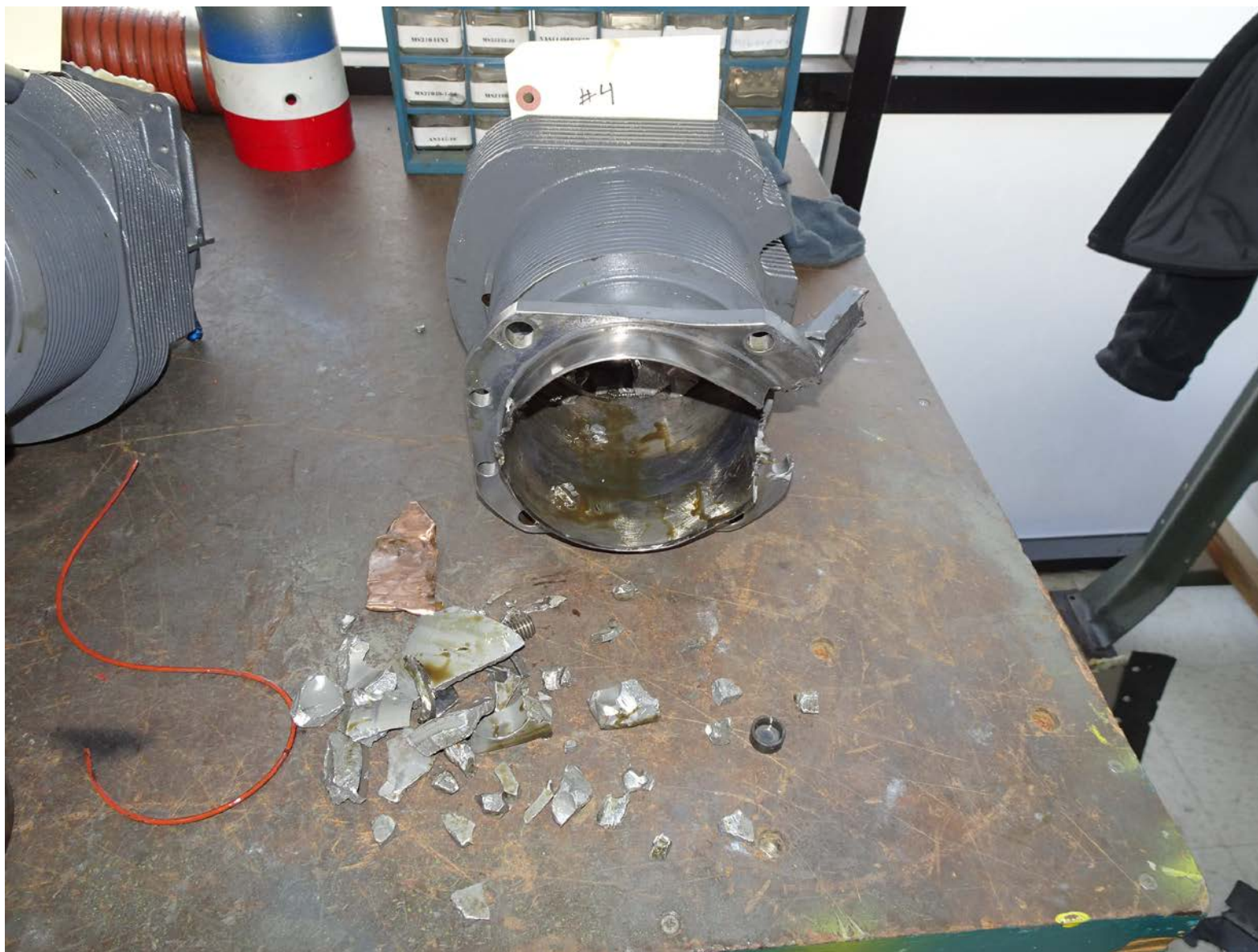
Photo 4 – View Cylinder No. 4 and Fragmented Parts (Courtesy of Piper Aircraft Company)
