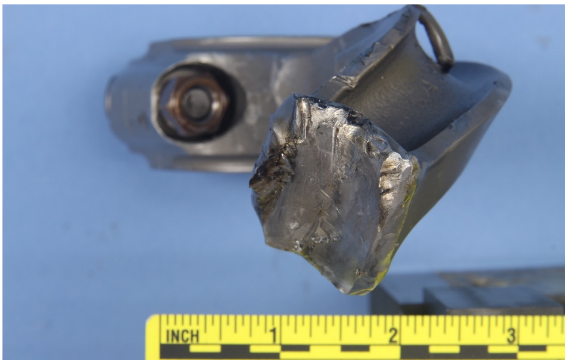
Figure 3 – View of the piston pin bore surface remnant on the connecting rod fragment.
