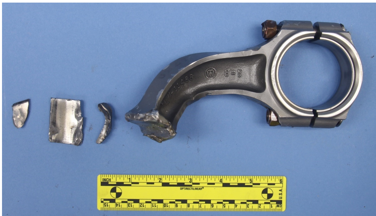
Figure 1 – The fragments of the connecting rod from the engine, as received.
