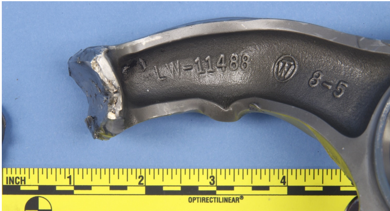
Figure 2 – The markings on the web of the connecting rod neck remnant.
