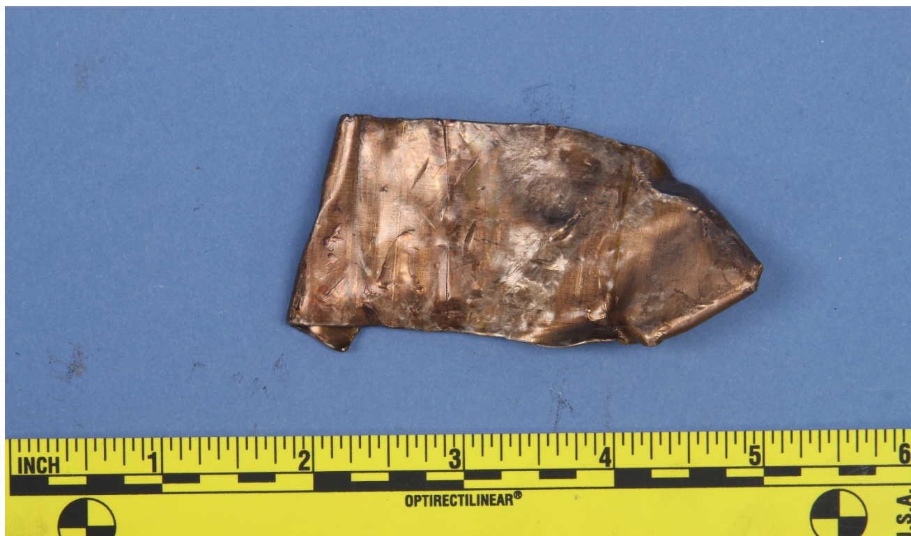
Figure 14 – The remainder of the bushing from the connecting rod pin bore, as received.
