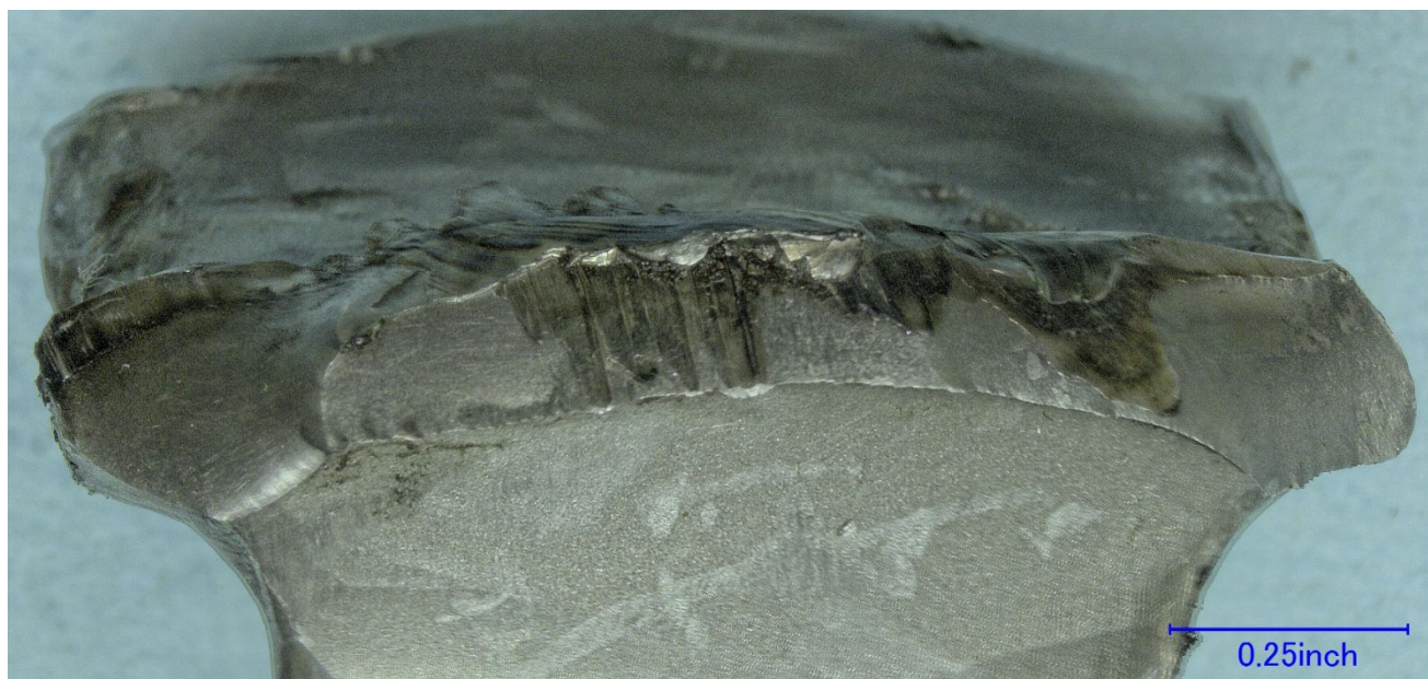
Figure 5 – The side of the connecting rod pin bore remnant, showing the fractured area with post-fracture batter and impact.
