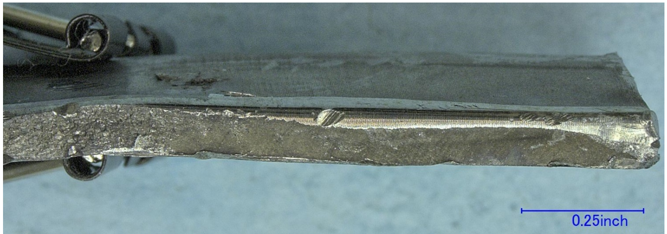
Figure 7 – View of the fracture surface of one of the smaller connecting rod pin bore remnants, showing crack arrest marks consistent with crack propagation from right to left.
