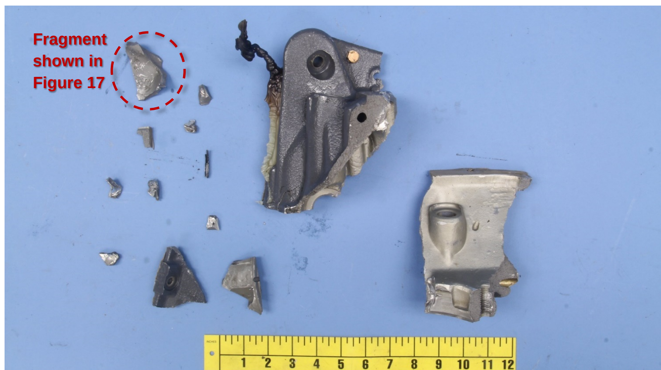
Figure 16 – Miscellaneous pieces of the housing submitted with the other engine parts.
